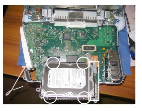
5. Remove four screws holding hard drive into bracket. Disconnect power and connector cables.
