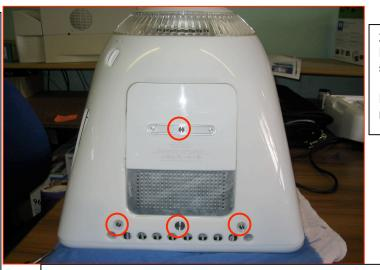
4. Remove processor board (9 screws). Unhook power button cable from the side, undo one plug near the top and four small plugs at the bottom before attempting to remove. Gently pull the processor board forward and lay it down.
