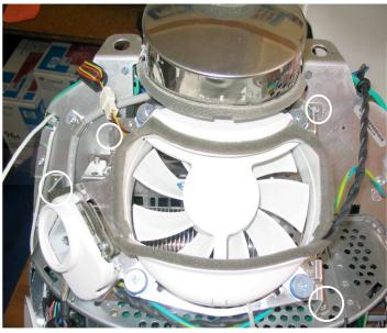
3. Remove fan and housing (4 screws). Do not fully disconnect fan and bracket, just hang off to the right, out of the way.
