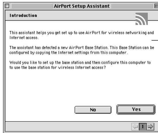
*The AirPort Setup Assistant screen that appears if a new AirPort Base Station is detected and the computer has never been set up to use AirPort. A different screen will appear if there are other networks in range or the computer has already been set up to use AirPort.*
