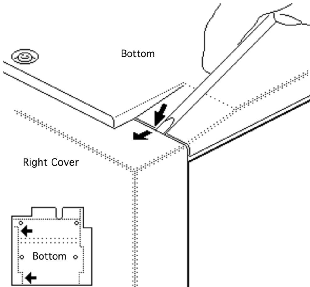
**Note:** Two hidden flex tabs on the bottom and two posts at the top attach the right cover to the feeder.
