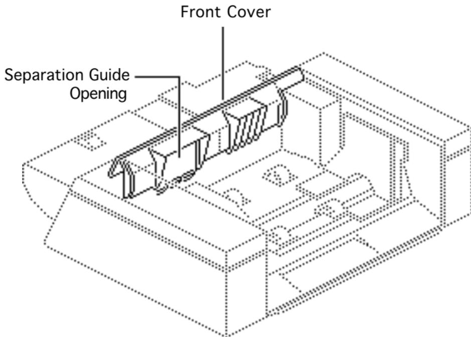
**Note:** If you have removed the separation guide plate from the front cover, you must adjust the gap between the separation guide plate and the primary feed roller.
