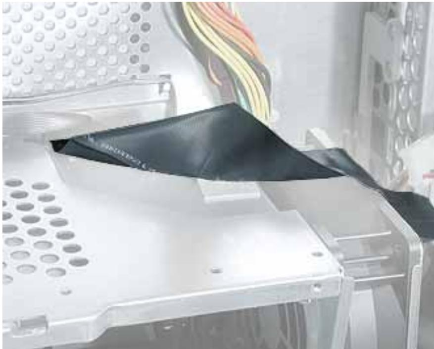
2. Open the two cable clamps at the bottom of the chassis.
