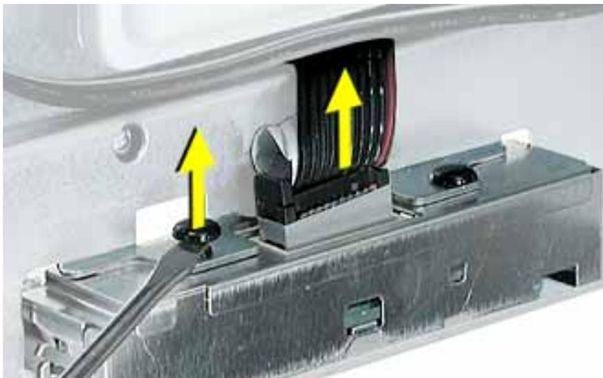
3. Using a #2 Phillips screwdriver, remove the front panel board mounting screw.
