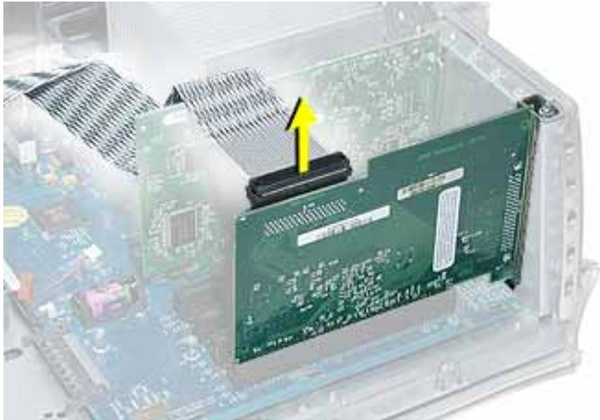
2. Disconnect the SCSI cable from the hard drives at the front and back hard drive carriers.
