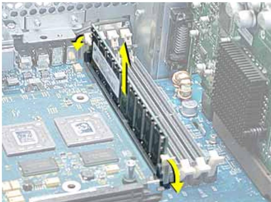
**Replacement Note:** The DIMM is designed to fit into the slot only one way. Be sure to align the notch in the DIMM with the small rib inside the slot.
