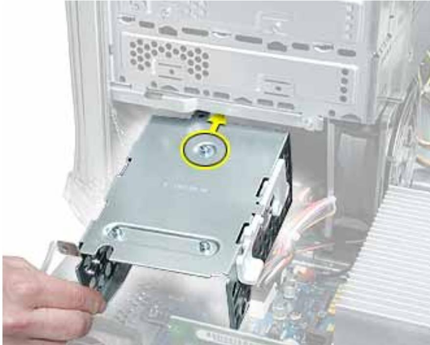
**Replacement Note:** Before closing the side access panel, make sure the P4 and P5 power cable connectors are either attached to the hard drives or tucked inside the front hard drive carrier.
