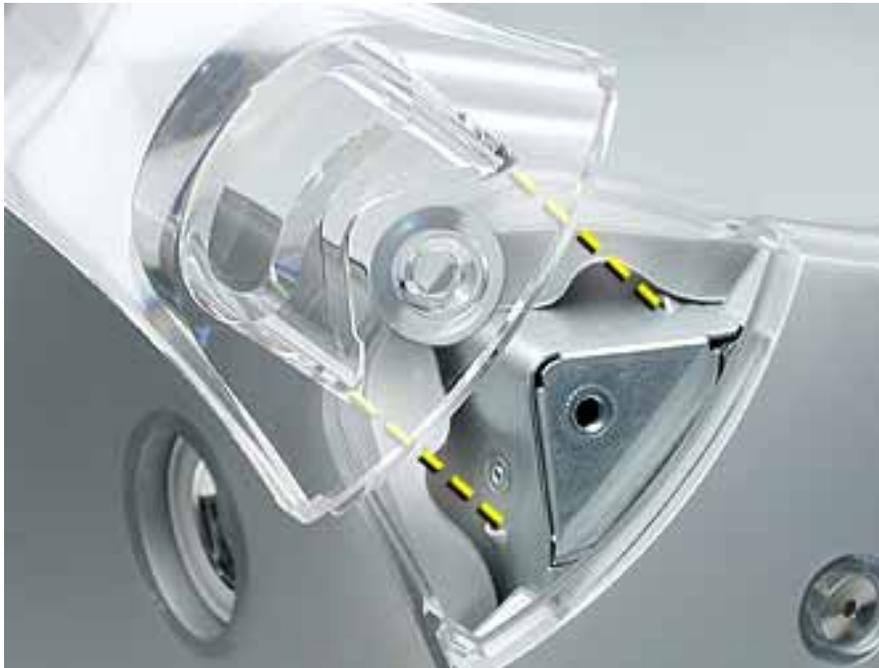
**Replacement Note:** When replacing a handle, make sure the inner prongs fit inside the raised points on the computer.
