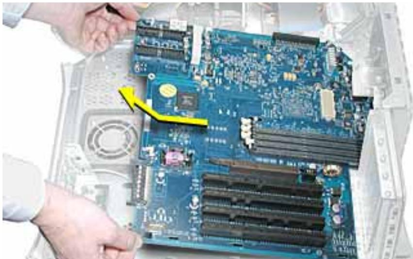
**Note:** After installing a replacement logic board, be sure to transfer the processor stiffener, processor, heatsink, DIMMs, and any other cards to the new board. You must also remove the battery insulator tab from the battery holder on the new board.
