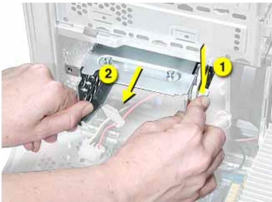
**Replacement Note:** Align the center mounting peg on the top of the carrier with the center channel on the underside of the optical drive shelf. This center peg helps to guide the carrier. Then align the two remaining pegs, and slide the carrier in until the pegs engage and the right side lever clicks into place.
