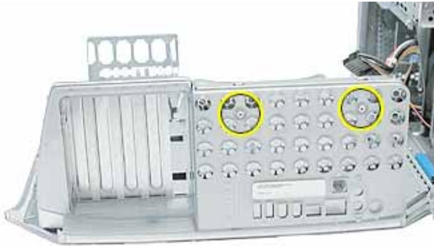
2. Remove the Phillips screw securing the access cover to the rear chassis. Remove the access cover.
