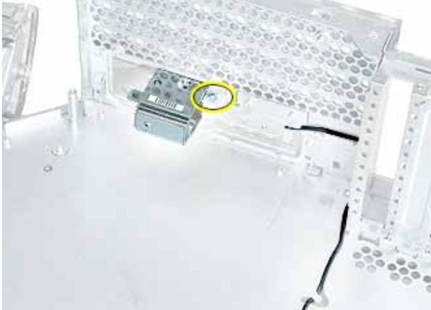
3. Swing the modem filter board out of the opening in the back chassis.
