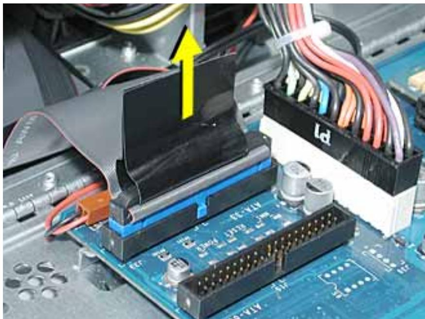
2. Using a small flat-blade screwdriver, gently lift up the locking tab on the lower fan cable and disconnect the cable from the logic board.
