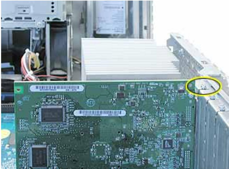
2. Gently hold back the clip on the video card connector to release the card.
