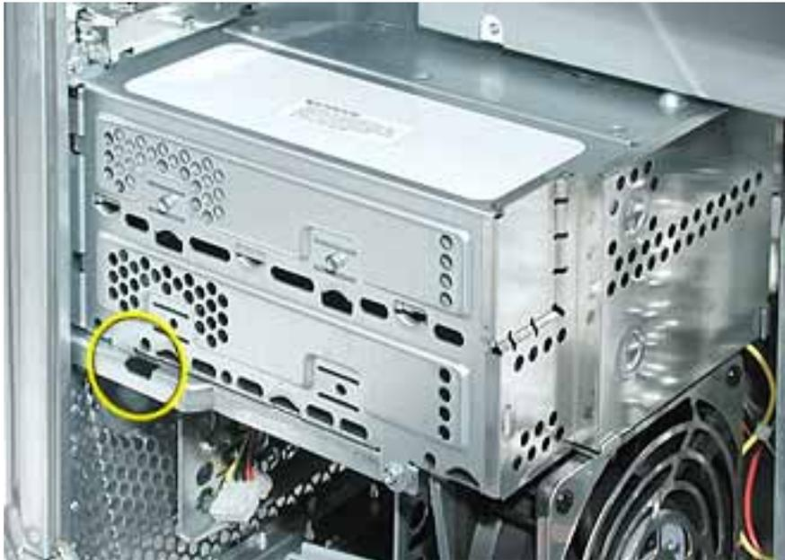
**Replacement Note:** Before sliding the rear panel back onto the carrier, make sure the top lip of the panel engages with the top edge of the drive carrier.
