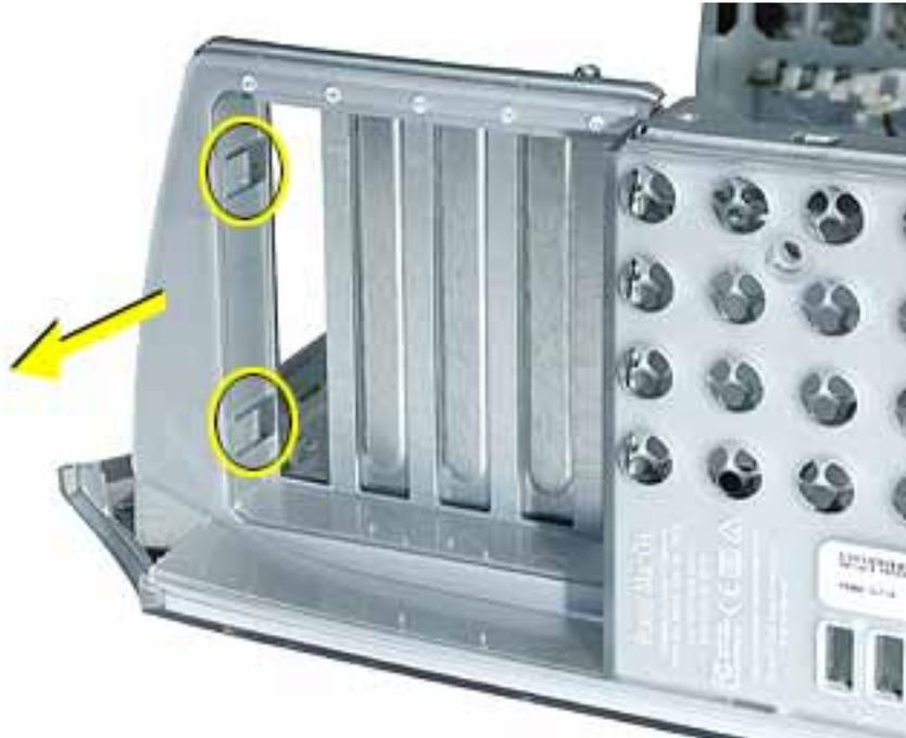
4. From inside the chassis, pry up the two tabs near the modem filter board.
