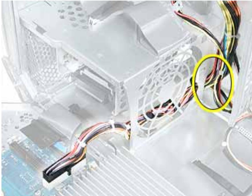
5. Slide the power supply forward and remove the power supply and cable harness from the computer.
