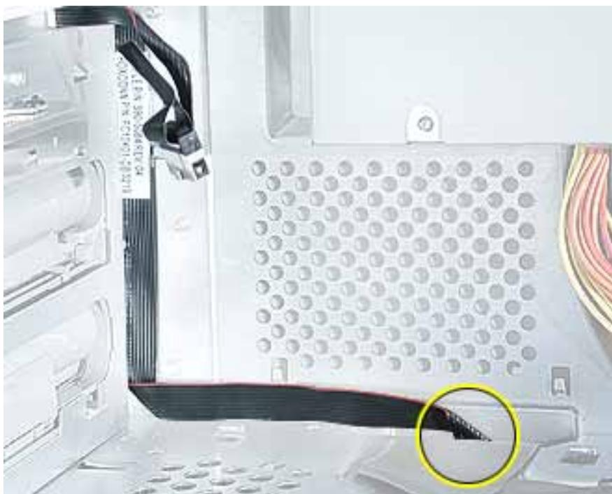
3. Open the two cable clamps at the bottom of the chassis and disconnect the front panel board connector from the logic board.
