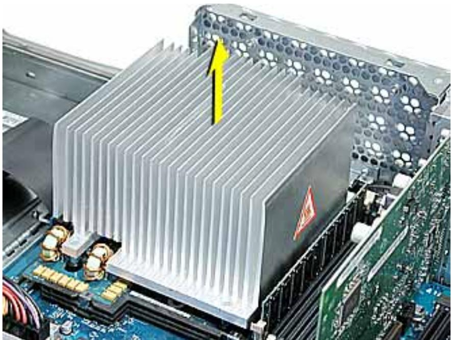
**Note:** Whenever you remove the heatsink, you must clean the heatsink base and add new thermal grease to the chips on the processor, as follows:
