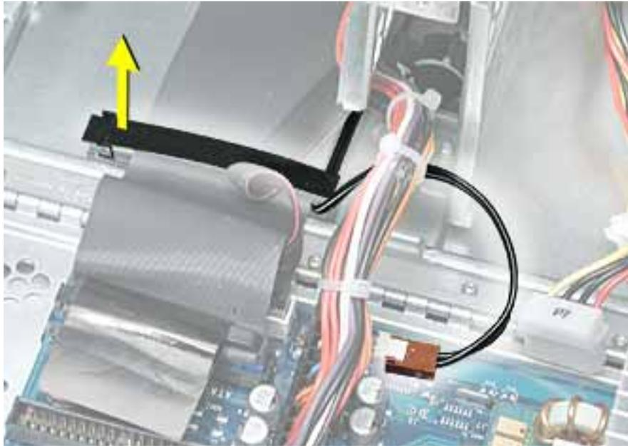
3. Route the cable up and out through the opening in the optical drive shelf and out from under the speaker case.
