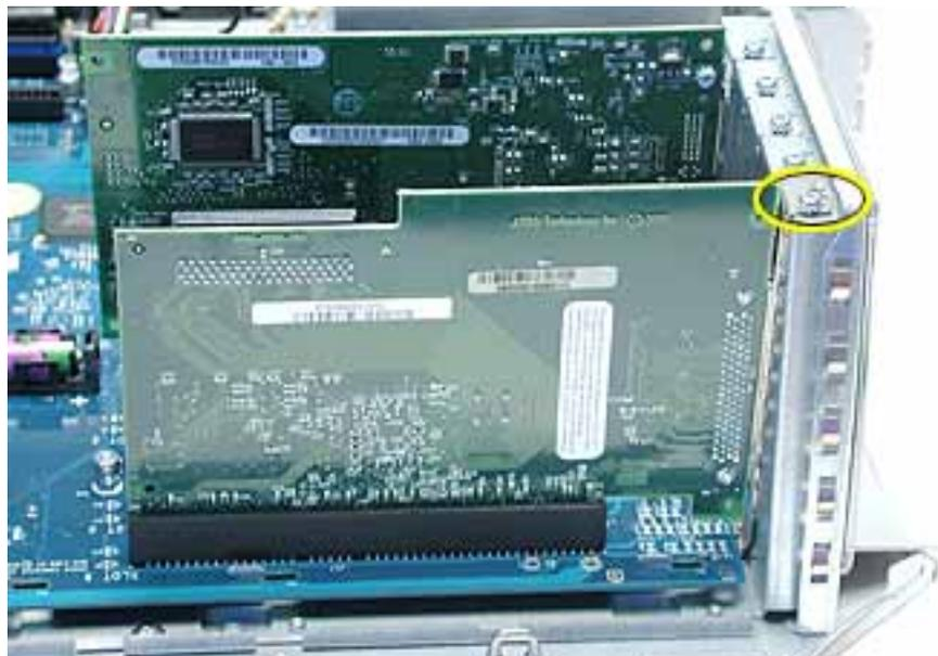
3. Lift up the SCSI card from the slot on the logic board.
