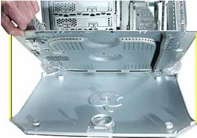
**Replacement Note:** When installing the replacement right side access panel, make sure the latch is closed, and the metal latch spring pin inside the chassis fits under the plastic latch tab, as shown.
