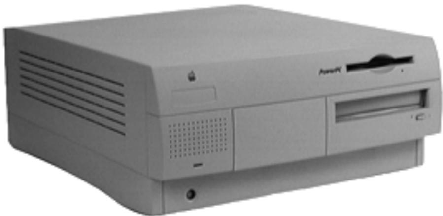
The Power Macintosh G3 desktop chassis design allows you to access the logic board and its components, including the removable processor, without having to remove the power supply or any drives. This flexible design makes this computer easy to service and upgrade.
