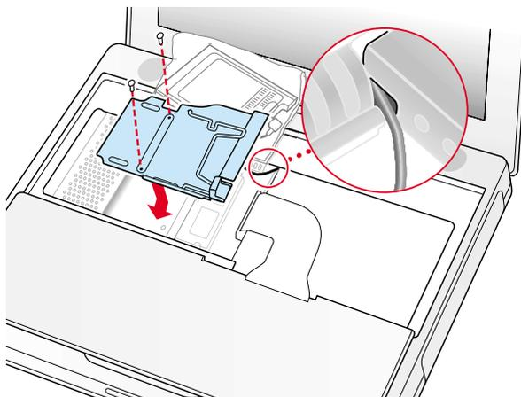
7. If you do not have an AirPort Card, flip down the wire holder over the AirPort Card antenna cable and secure it by inserting the prongs of the holder into the slots in the RAM shield (**Figure 11**).
