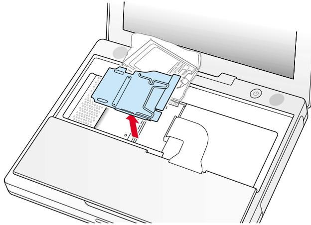
6. Locate the keyboard cable connector (**Figure 9**).
