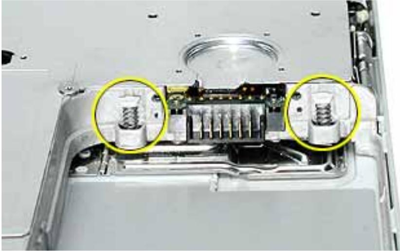
**Note:** When reassembling the computer, make sure that the two springs in the battery connector are in place before installing the bottom case. Each spring has a plastic cap on one end. The cap should fit securely on the spring, and the curved side of the cap should be positioned against the inner frame.
