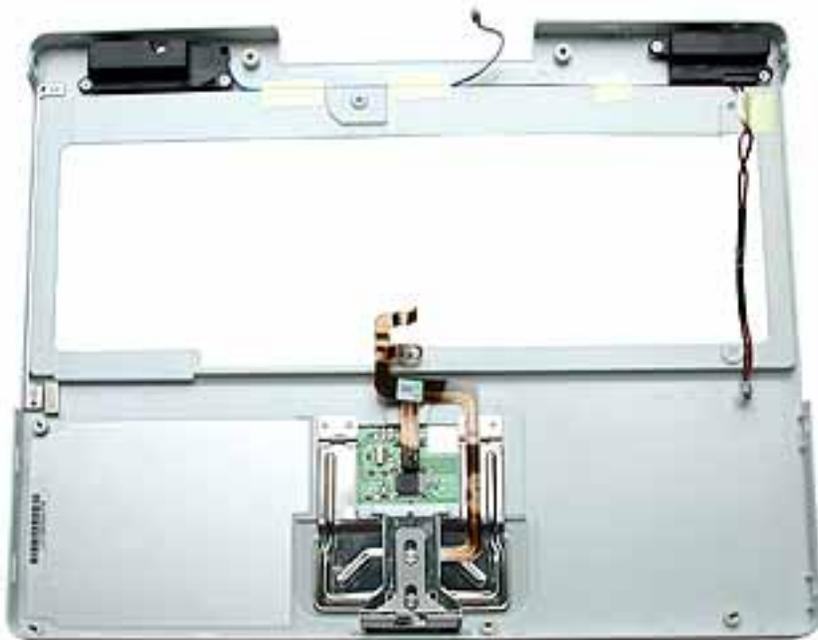
16. Install the replacement top case, and reassemble and test the computer.
