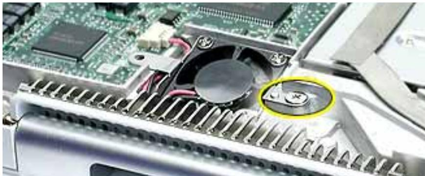
2. Lift the fan and bracket from the computer, and use a black stick to disconnect the connector from the logic board.
