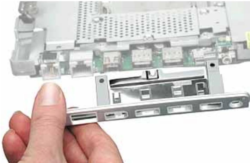
3. Install the replacement I/O bezel, and reassemble and test the computer.
