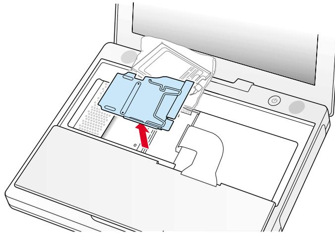
6. Locate the installed memory card and brackets that secure the card on both sides (**Figure 9**).
