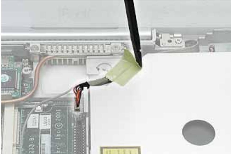
4. Remove the screw securing the flat section of the LVDS cable.
