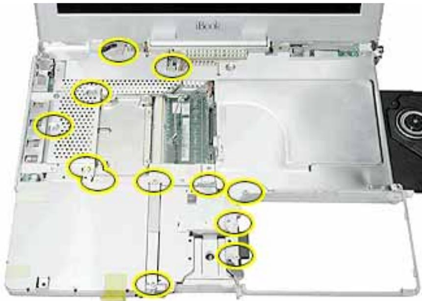
2. Using a black stick, carefully peel up, but do not remove, the two foil strips and three pieces of tape.
