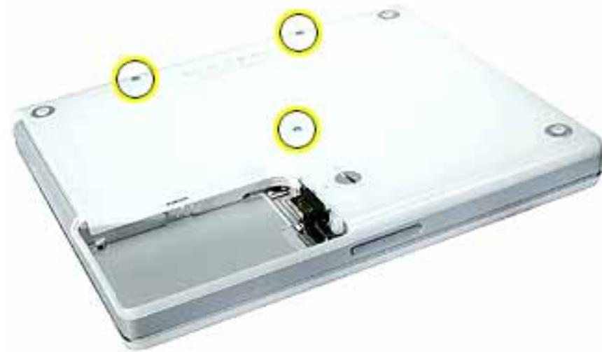
3. Using a black stick, peel up the three rubber feet from the metal sockets.
