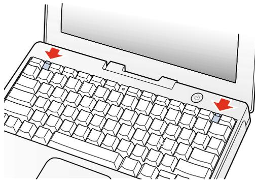
5. Let go of the keyboard release tabs to secure the keyboard in place.
