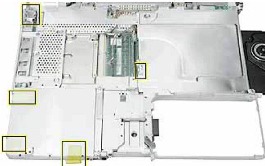
3. **Warning: Do not bend the top shield.** Lift the top shield off the computer, being careful where it might catch on the highlighted areas shown.
