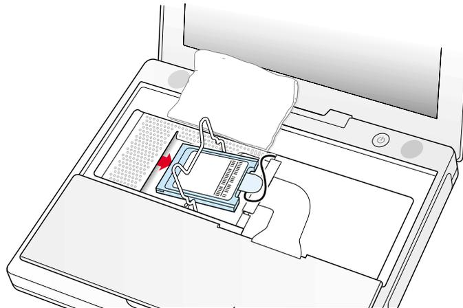
3. If an AirPort Card is not installed, unlatch the flexible wire holder to release the AirPort Card antenna cable.
