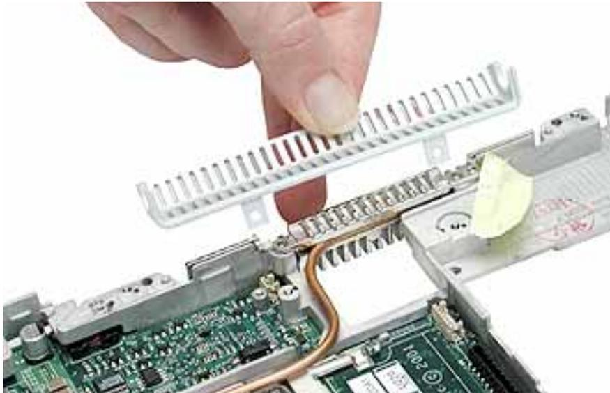
5. Remove the remaining screw at the heat spreader plate.
