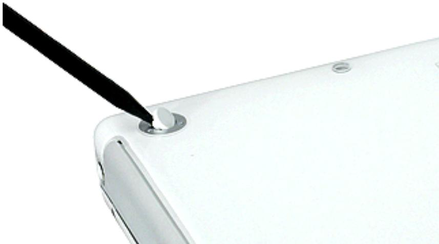
4. Remove the three Phillips screws from the metal sockets.
