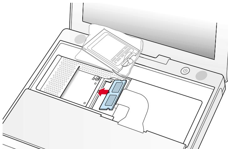
2. Gently push the top of the card down until the brackets snap onto both sides of the memory card to lock it into place (**Figure 11**).
