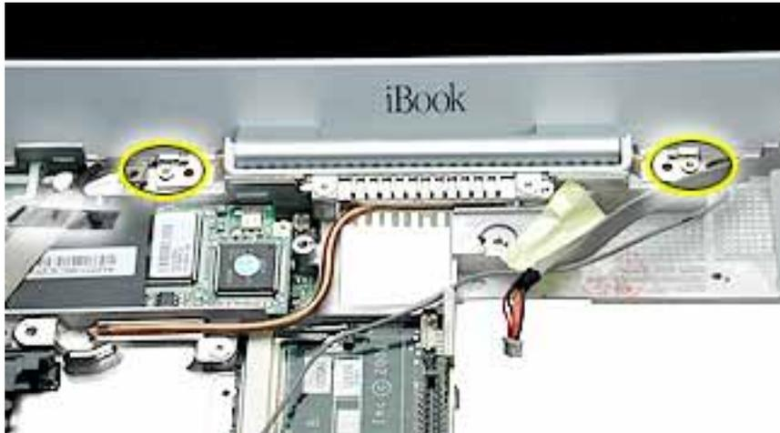
6. **Warning: When lifting the display, be careful not to strain the cables.**
