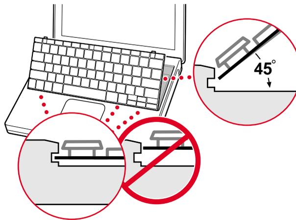
4. Pull down on the keyboard release tabs and then press down on the top portion of the keyboard (**Figure 16**).
