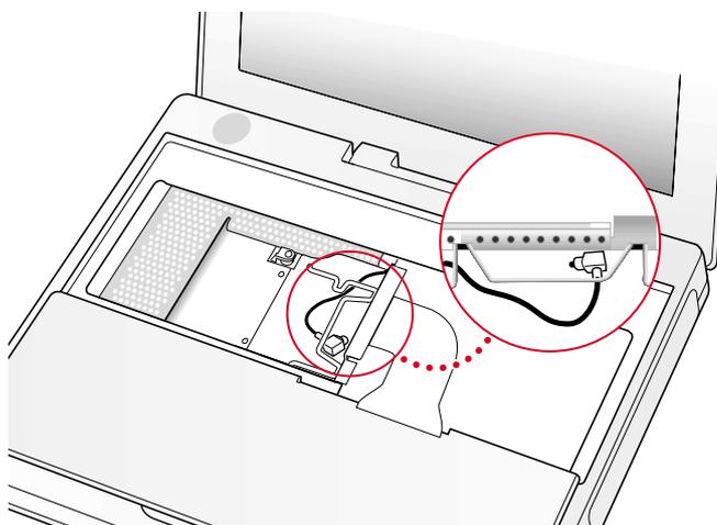
8. If you have an AirPort Card, gently slide it (with the AirPort ID number and bar code facing up) under the wire bracket and securely into the AirPort Card slot.
