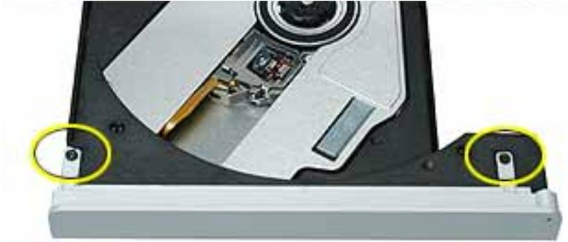
2. Gently tilt the door away from the screw holes to release the hooks underneath that hold the door in place.
