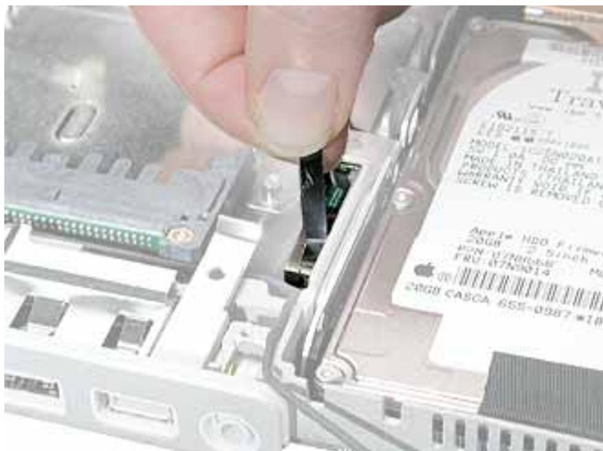
3. Remove the screw securing the flat section of the LVDS cable.
