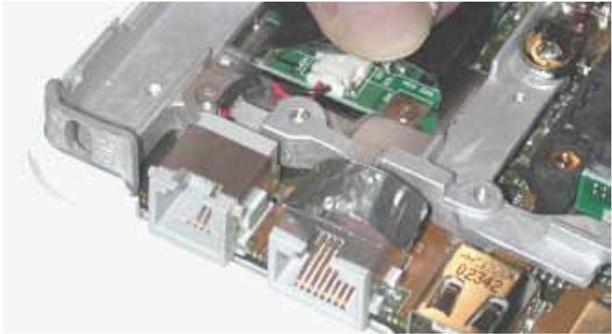
4. Slide the modem port forward and off of the logic board.
