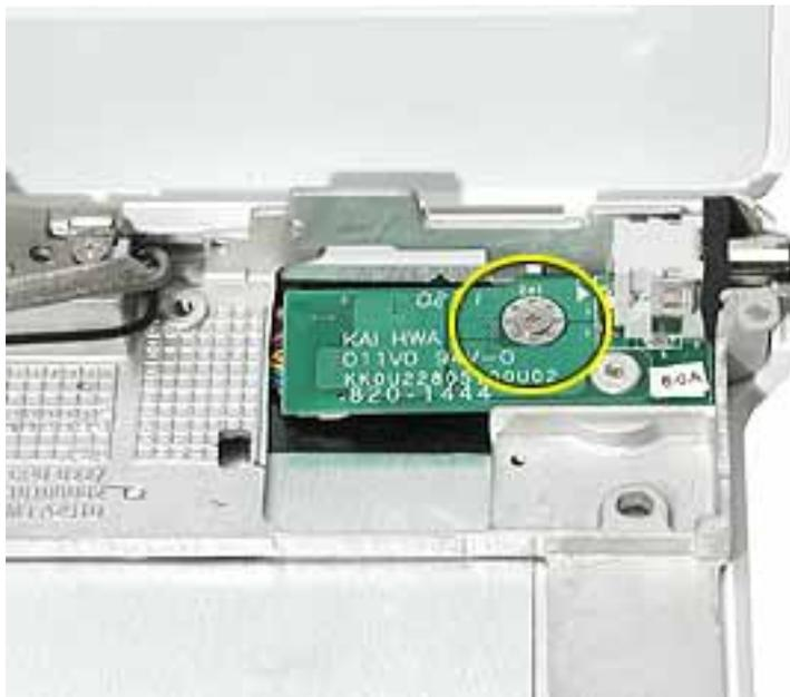
2. Tilt up the DC board, and use a black stick to disconnect the cable connector from the DC board.
