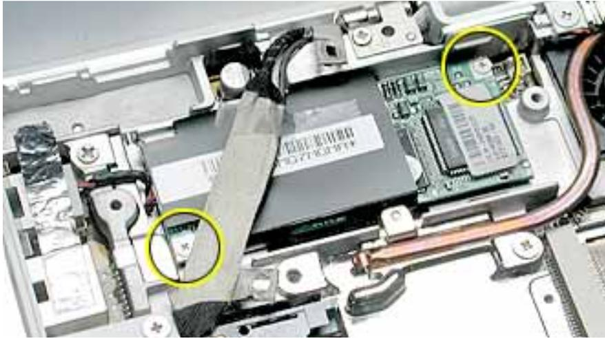
3. Tilt up the end of the modem to disconnect it from the logic board.
