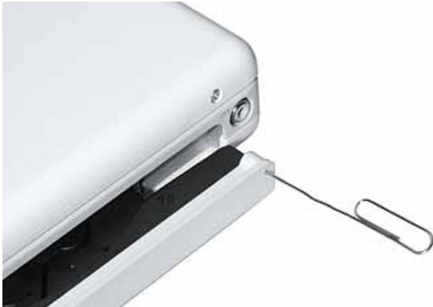
8. **Warning: Avoid pressure on the optical drive tray. When removing the optical drive bezel, putting pressure on the drive tray can damage the drive.**
