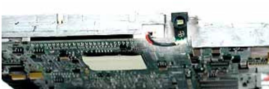
2. Using a black stick, disconnect the sleep light board connector from the logic board.
