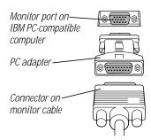
If you installed a graphics card in your computer, connect the monitor cable to the graphics card's port instead. For information about installing graphics cards, see the manual that came with your computer or graphics card.
