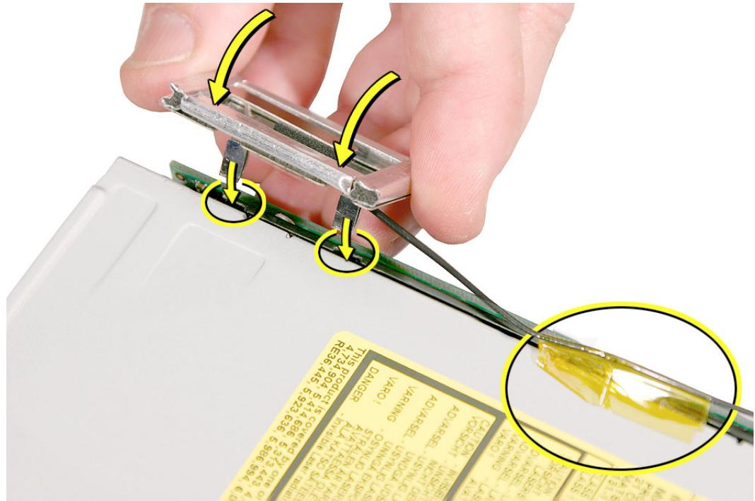
25. Fasten the AirPort Extreme antenna onto the internal frame. The antenna is held in place by the black clip. **Note:** If you are performing an upgrade, secure the antenna cable with kapton tape.
