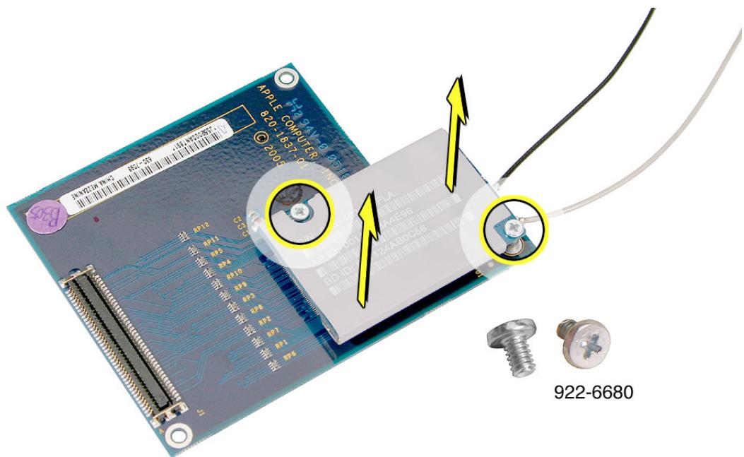
17. Disconnect the antenna(s) from the AirPort Extreme/Bluetooth card. The silver cable is for Bluetooth and the black cable is for AirPort Extreme.
