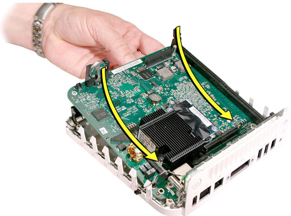
4. Gently push the LED away from the board as you lower the board into the bottom housing. **Note:** Don't bend the LED too much or it could snap off the bottom housing.
