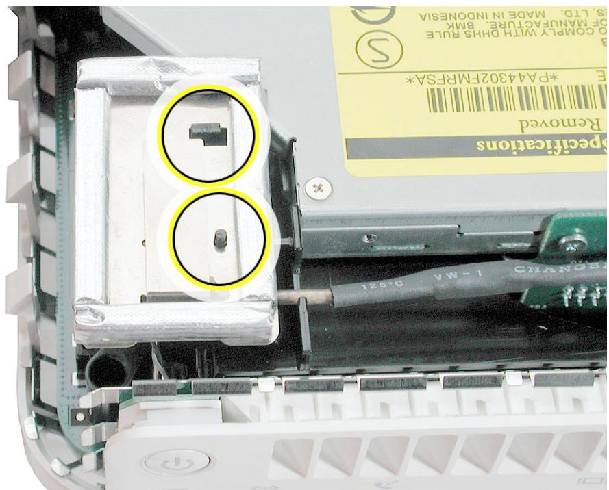
12. Secure the power button cable to the internal frame with the kapton tape.
