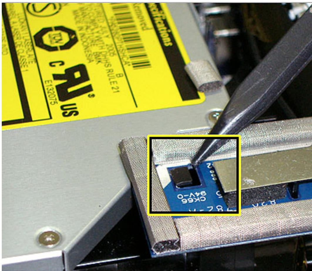
16. Secure the power button cable to the internal frame with the kapton tape.
