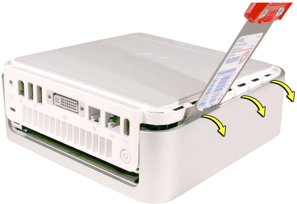
7. Push the I/O panel upward until the top housing is removed. The popping sounds will continue as you push the I/O panel; this is normal.
