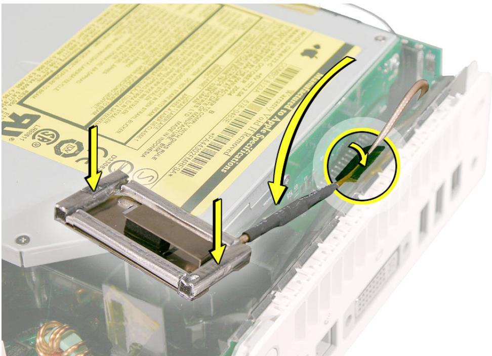
8. Gently fasten the antenna onto the internal frame. The antenna is held in place by the black clip and black post (shown below).
