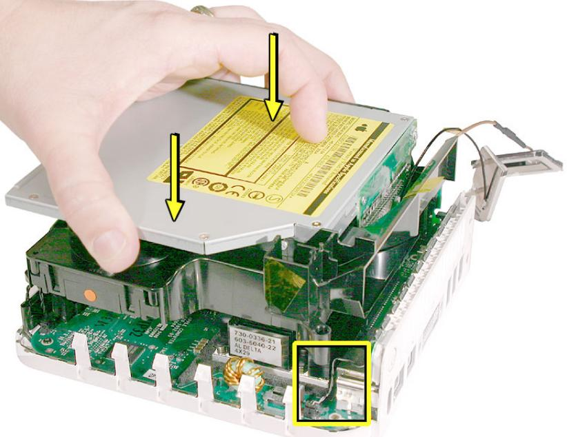
4. Route the antenna cables to the right side of the interconnect board on the internal frame as you continue lowering the internal frame onto the logic board.
