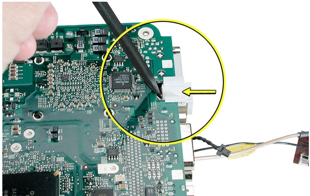
3. Reinstall the logic board into the bottom housing. Line up the ports on the board with the openings on the bottom housing.
