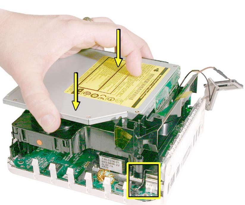
7. Route the antenna cables to the right side of the interconnect board on the internal frame as you continue lowering the internal frame onto the logic board.
