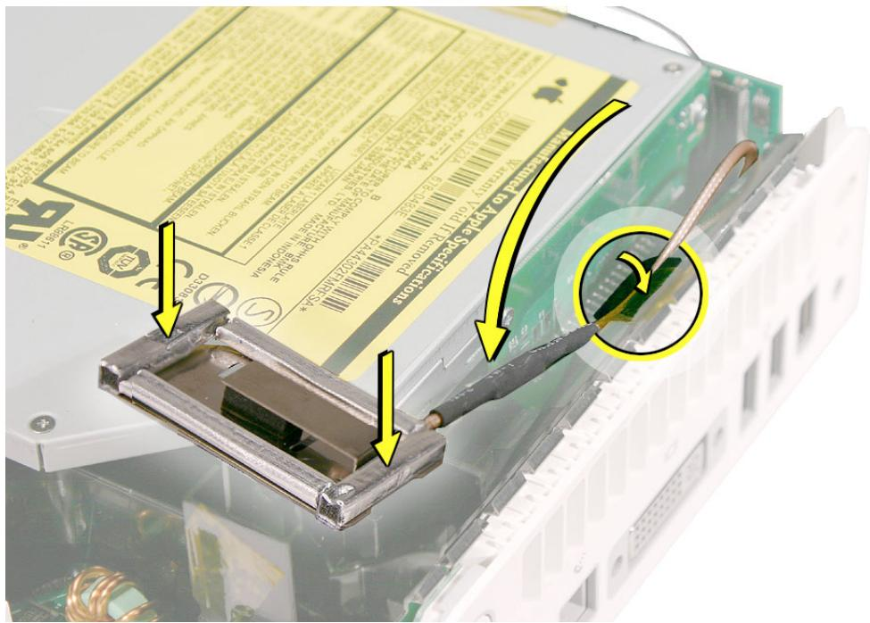
18. Gently fasten the antenna onto the internal frame. The antenna is held in place by the black clip and black post (shown below). Attach additional kapton tape to the internal frame to hold the AirPort antenna in place (if necessary).
