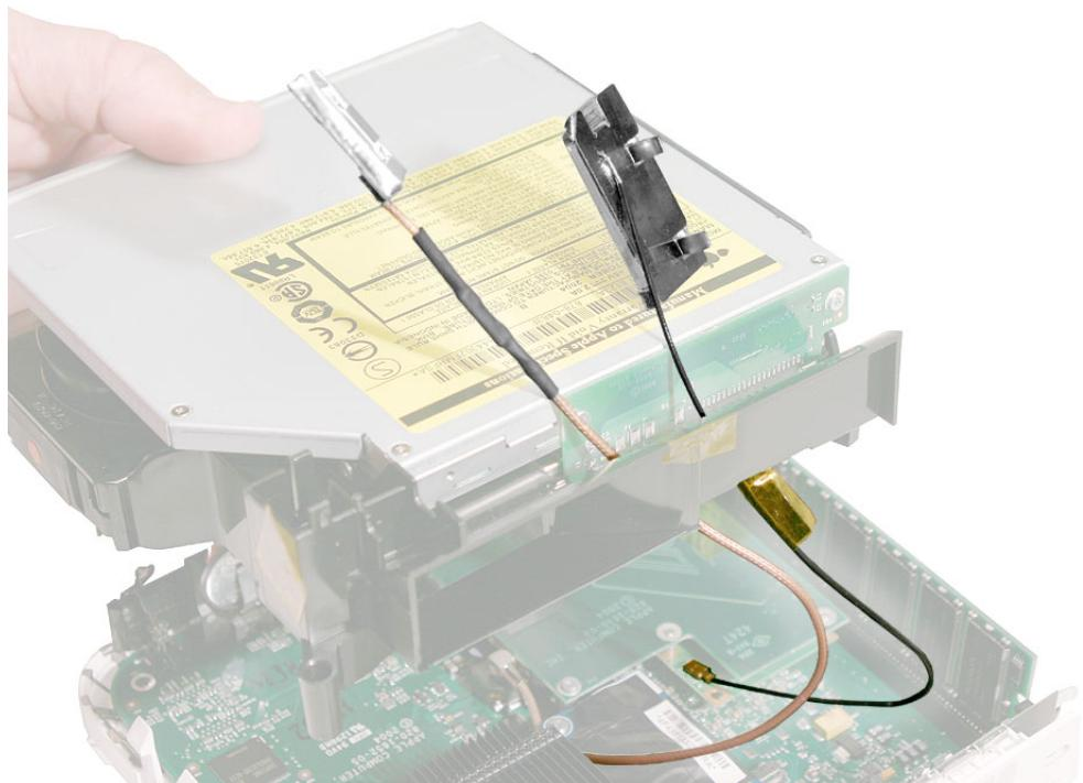
21. Lower the internal frame into place.
