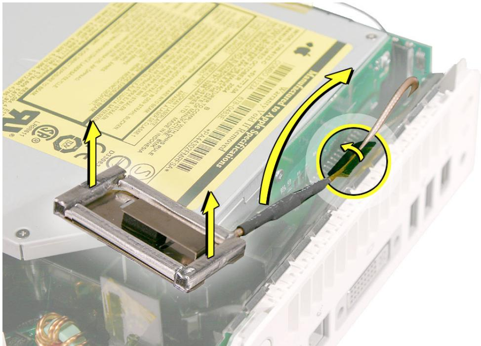
5. Set the AirPort antenna off to the side. **Note:** The AirPort Extreme card and antenna cable are connected to the mezzanine board located under the internal frame.
