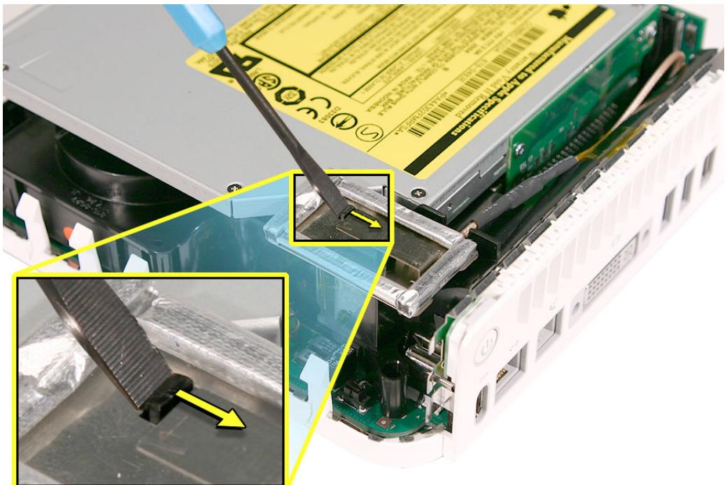
4. Carefully lift the antenna up and off the internal frame. Free the antenna from the kapton tape (circled). **Important:** Take care handling the AirPort antenna as a bent or warped antenna will affect Airport connectivity.
