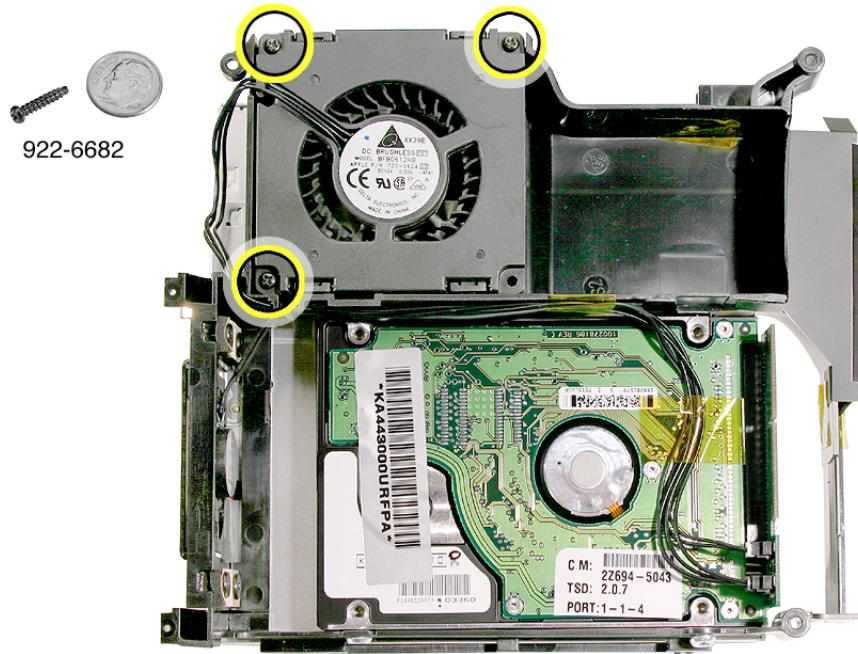
2. Free the fan cable from the clip on the internal frame.
