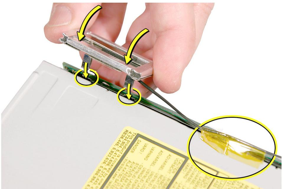
9. Replace the AirPort Extreme antenna. Secure the cable with kapton tape.
