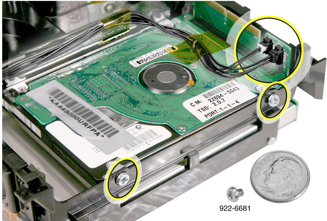
4. Replace the two hard drive screws on the inside of the internal frame.
