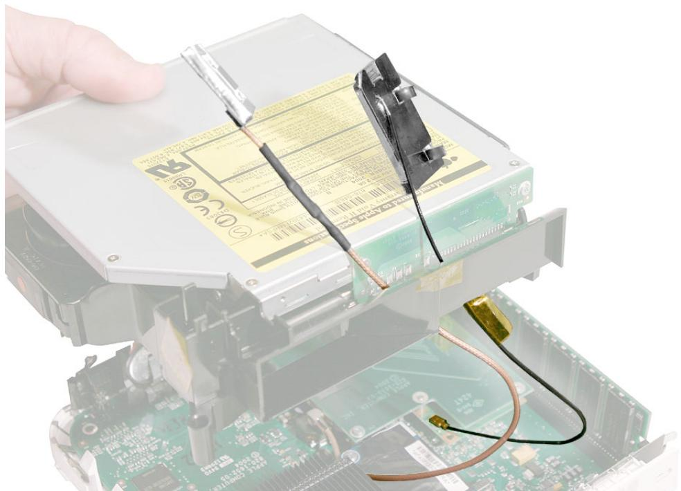
13. Lower the internal frame into place. **Note:** Route the power button cable out of the way of the internal frame.
