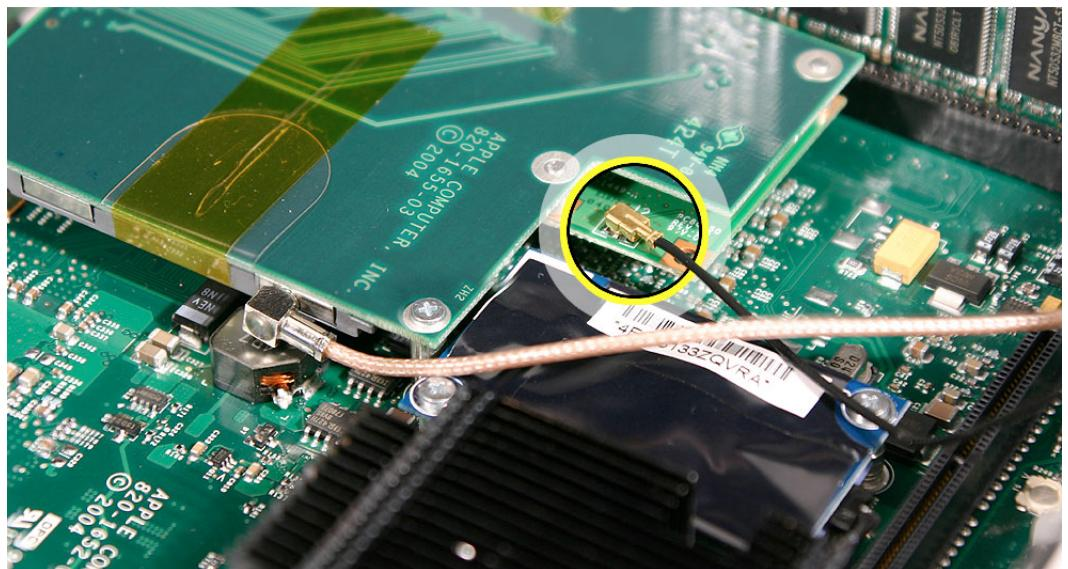
13. Remove the two screws on the mezzanine board. Lift the mezzanine board straight up and off the logic board connector. **Caution:** The AirPort antenna cable is still attached to the mezzanine board. Remove the AirPort antenna cable if required to perform the repair.
