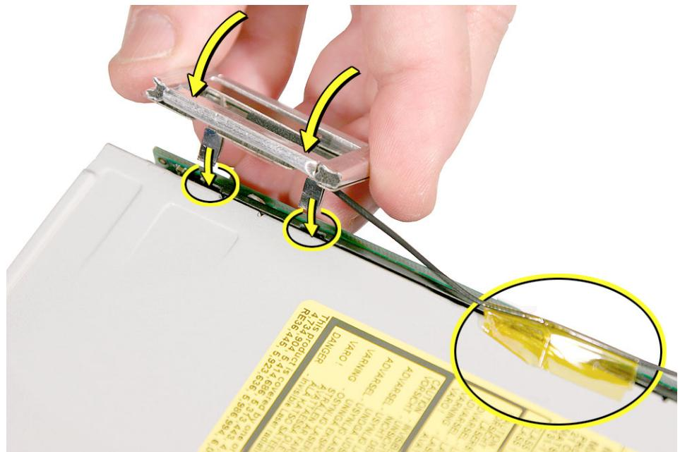
10. Replace the AirPort Extreme antenna and secure the cable with kapton tape.
