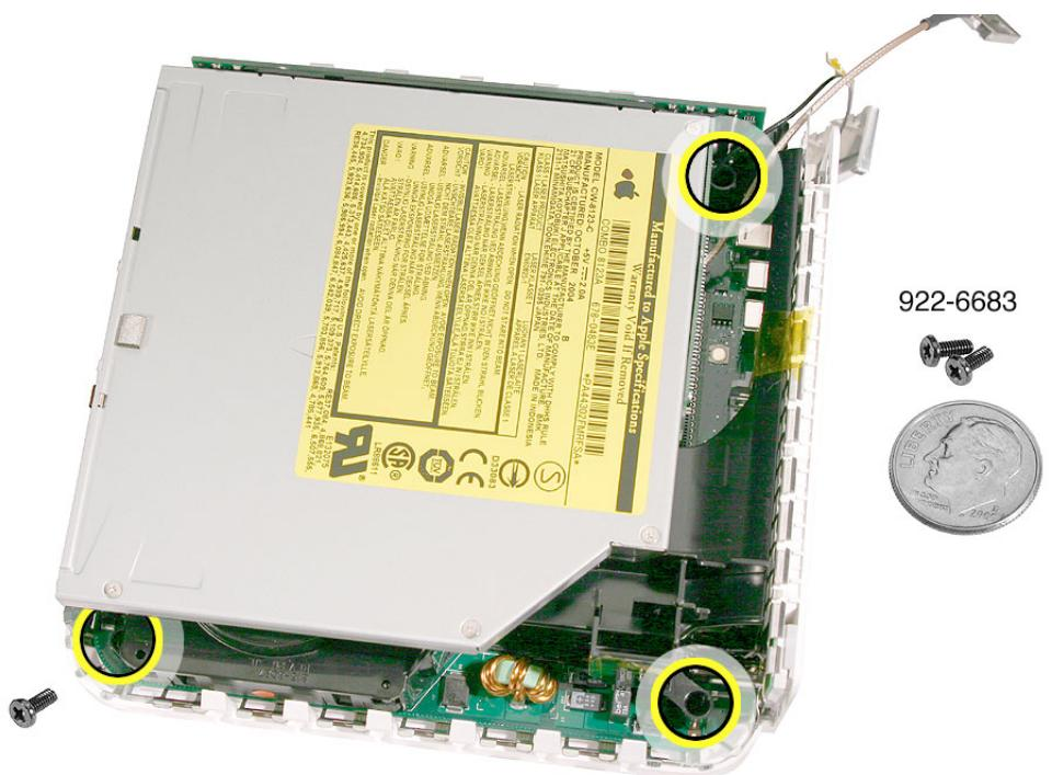
8. Lift the internal frame straight up.
