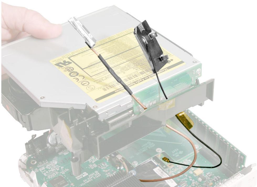
6. Lower the internal frame into place. **Note:** Route the power button cable out of the way of the internal frame.
