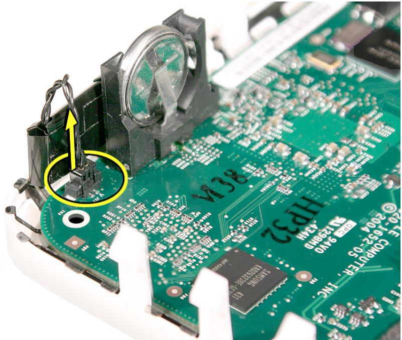
4. After disconnecting the LED cable, gently push the LED away from the board to free the logic board from the bottom housing. **Note:** Don't bend the LED too much or it could snap off the bottom housing.
