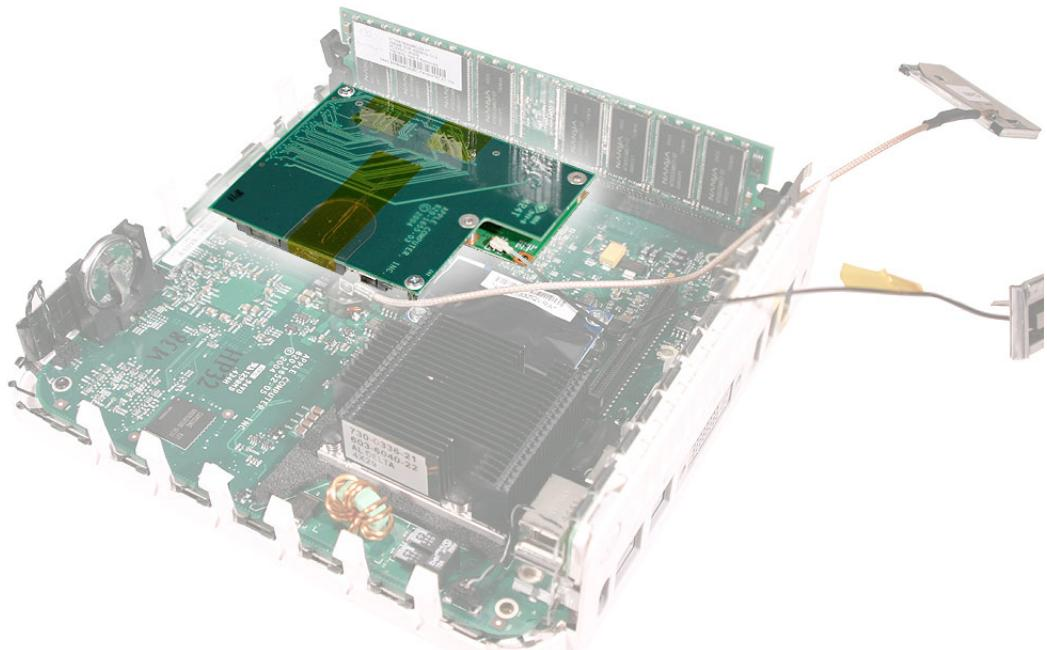
4. Reassemble the computer and test. If the Bluetooth board is still not recognized, test with a known good Bluetooth board. If the known good board is recognized, replace the Bluetooth board or the AirPort/Bluetooth combo card on the new Mac mini.
