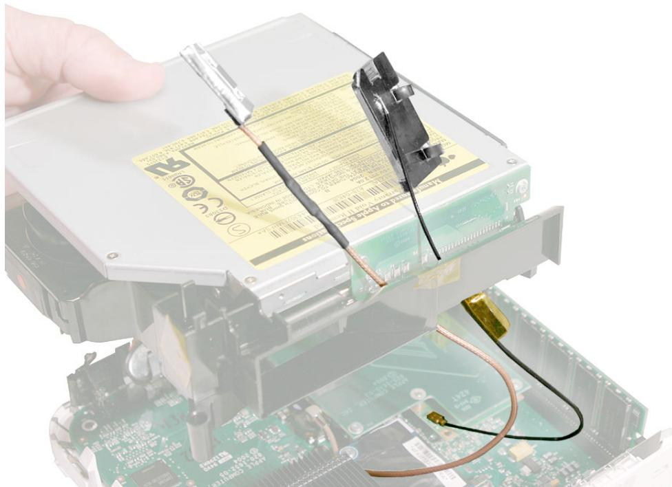
5. Lower the internal frame into place. **Note:** Route the power button cable out of the way of the internal frame.
