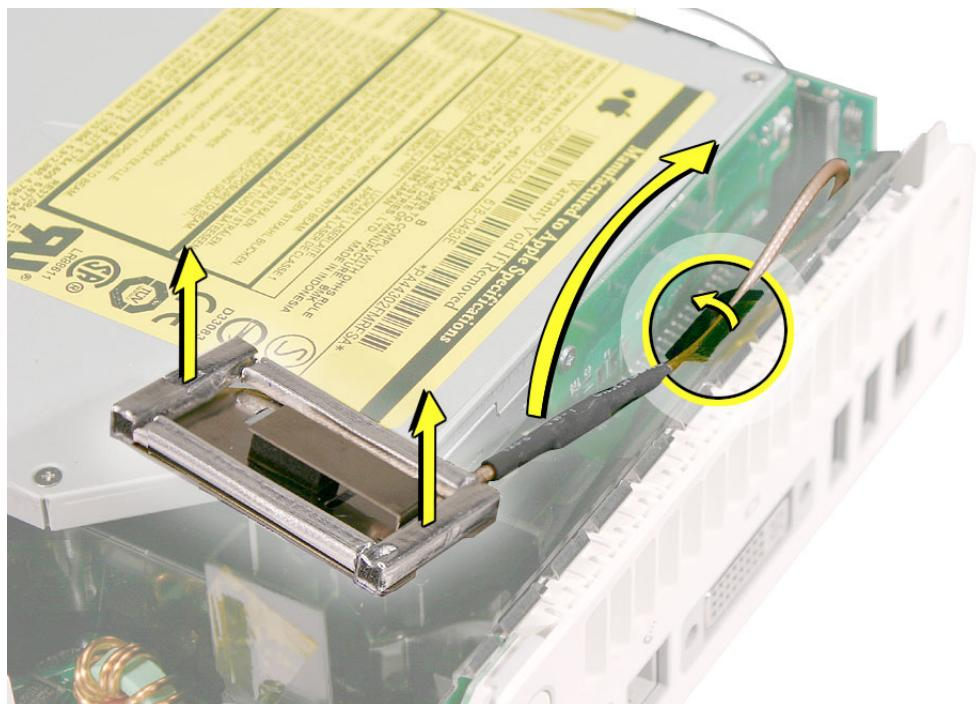
8. Set the AirPort antenna off to the side. **Note:** The AirPort card and antenna cable are connected to the mezzanine board located under the internal frame.
