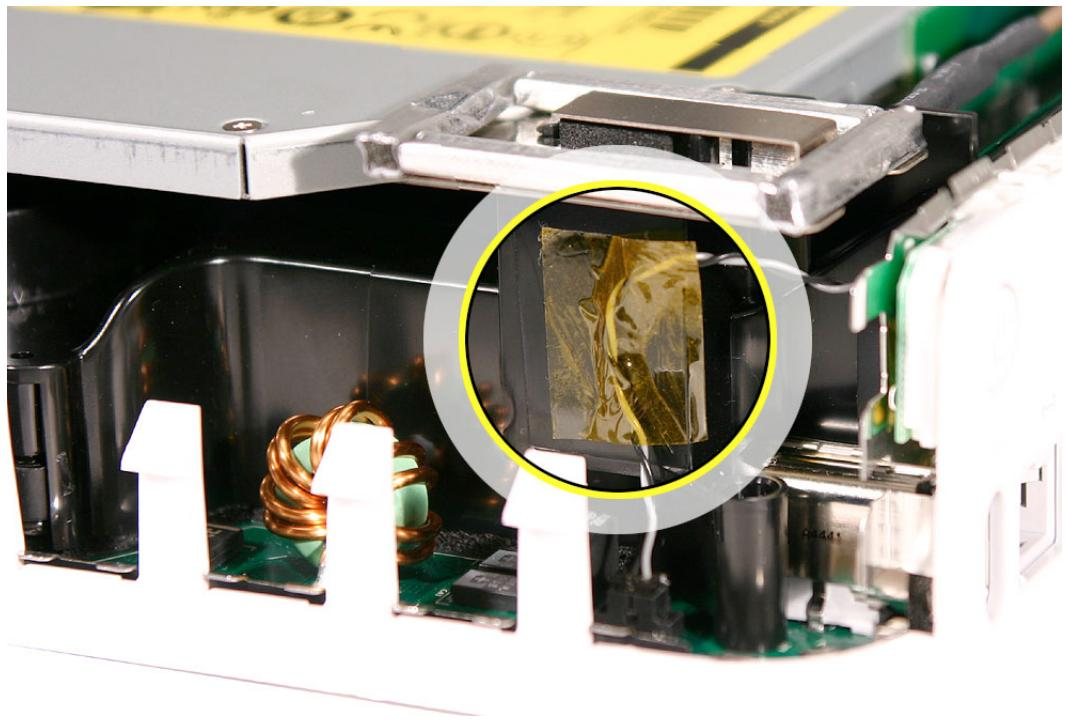
15. Lift the internal frame straight up and set it aside.
