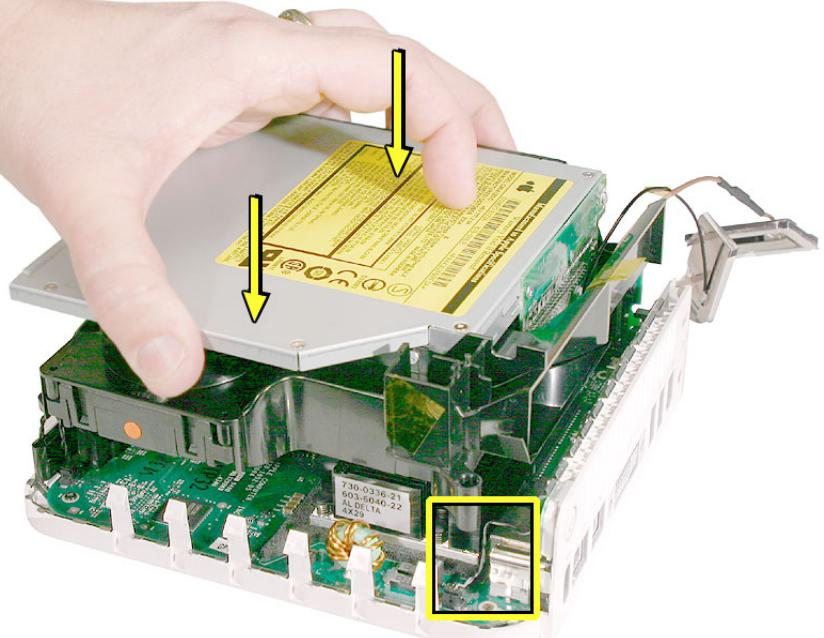
6. Route the antenna cables to the right side of the interconnect board on the internal frame as you continue lowering the internal frame onto the logic board.
