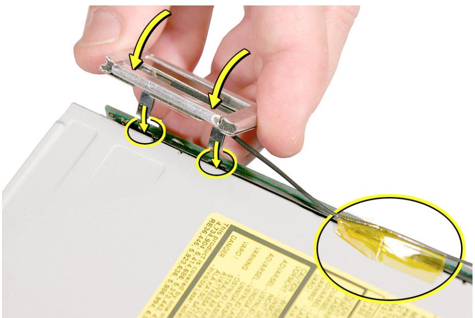
17. Replace the AirPort Extreme antenna. Secure the cable with kapton tape. **Important:** Take care handling the AirPort antenna as a bent or warped antenna will affect AirPort connectivity.
