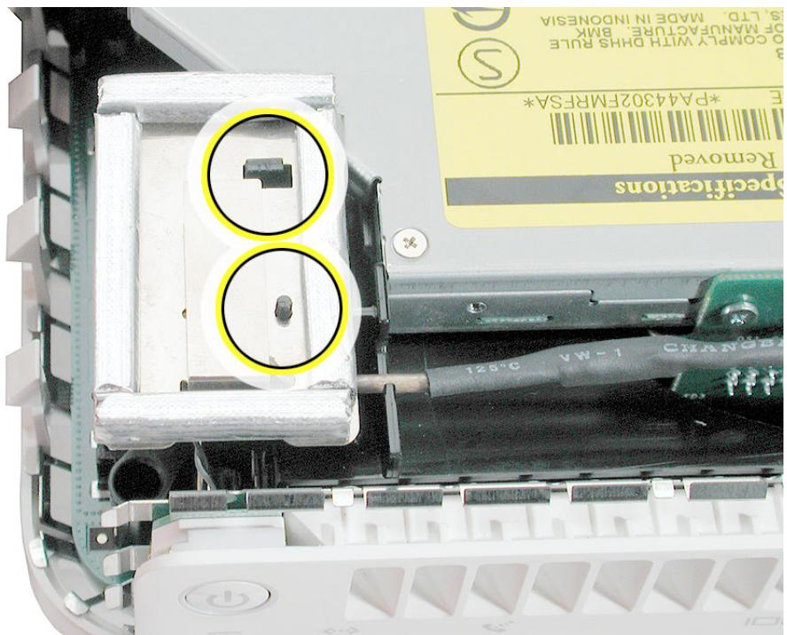
27. **Note:** If the airport antenna board contained in the finished goods upgrade kit has too large a hole (shown below) for the internal frame to clip onto, use additional kapton tape to secure the antenna to the internal frame. Either place a little kapton tape beneath the antenna board or place a strip of tape next to and running parallel to the antenna board, going from the optical drive across to the internal frame, securing the antenna cable to the internal frame.
