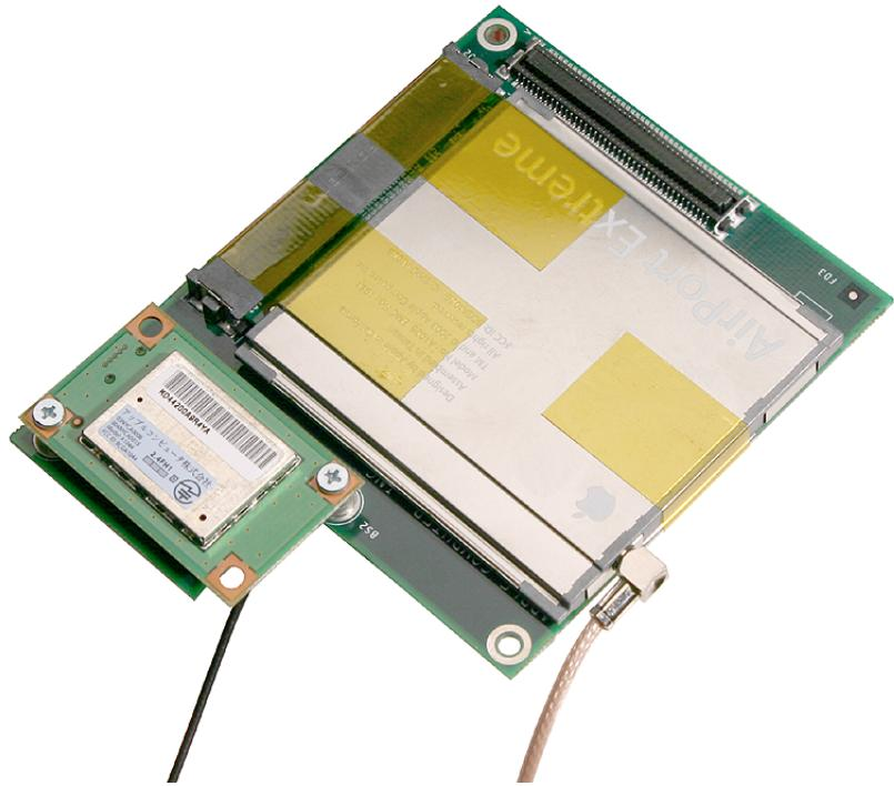
17. Turn over the mezzanine board so the AirPort Extreme card is facing down. Connect the mezzanine board to the connector on the logic board. Install the two screws on the mezzanine board.
