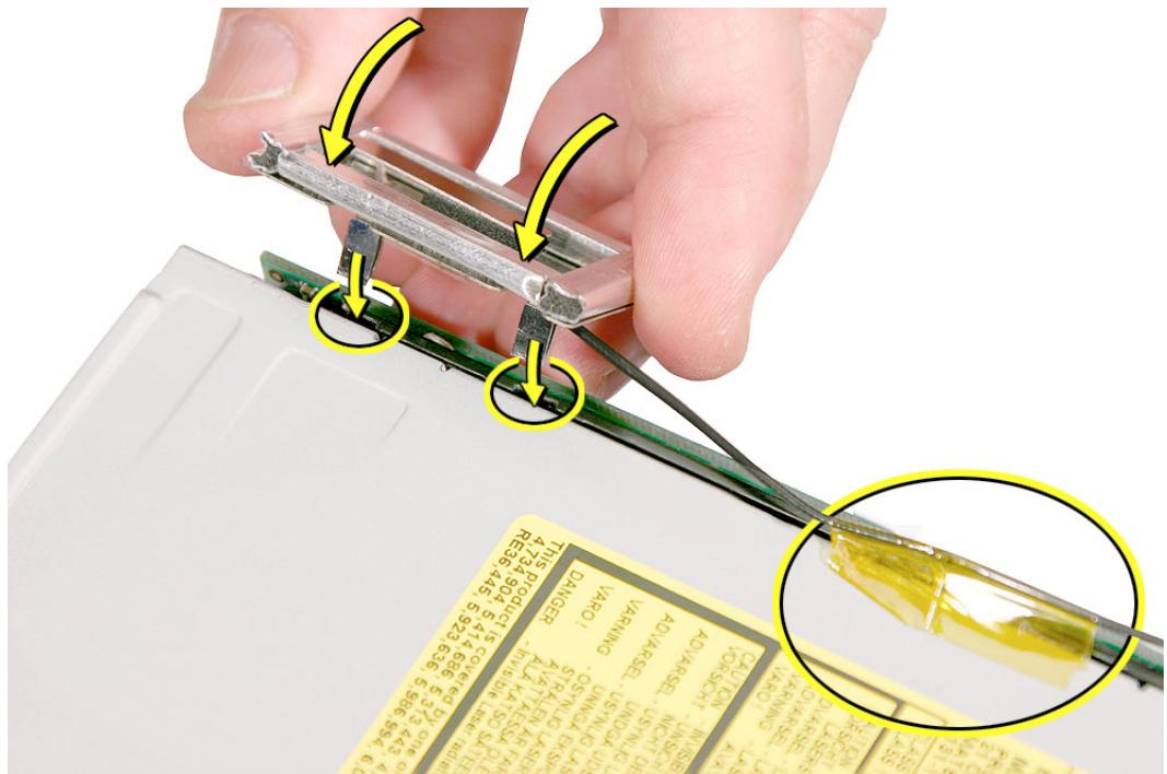
13. Fasten the AirPort Extreme antenna onto the internal frame. The antenna is held in place by the black clip. **Note:** If you are performing an upgrade, secure the antenna cable with kapton tape.
