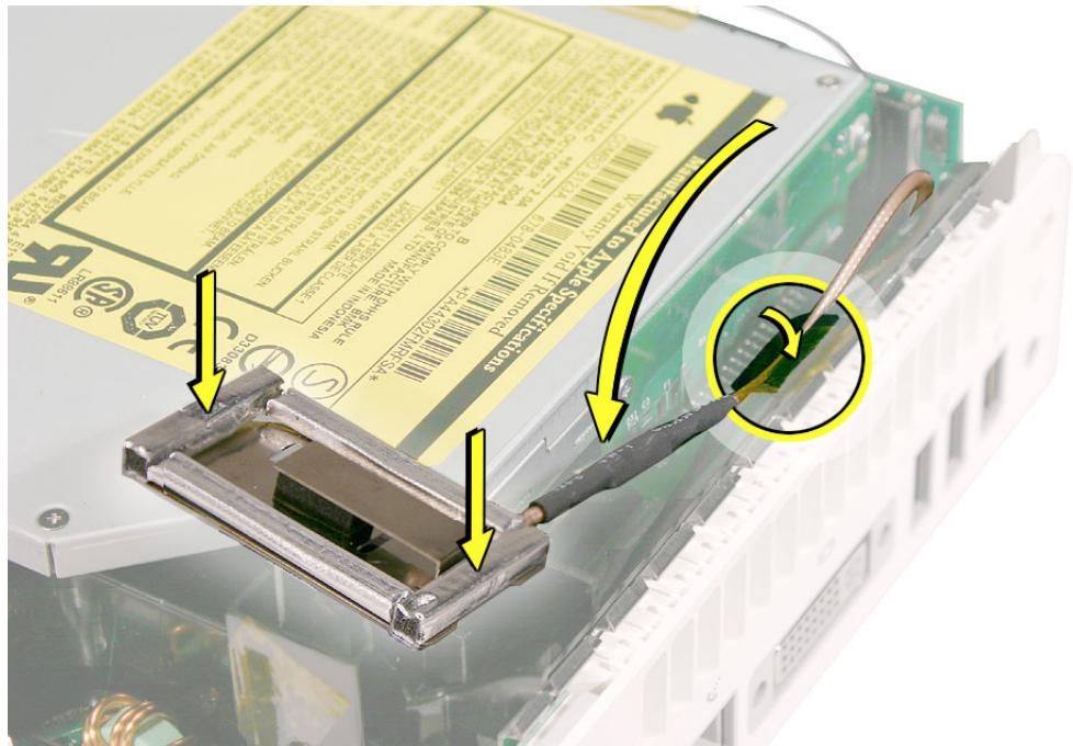
26. Lower the AirPort Extreme antenna over the black post and the clip (circled below) on the internal frame.
