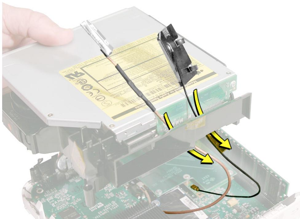
12. The following parts are connected to the internal frame (black plastic):
