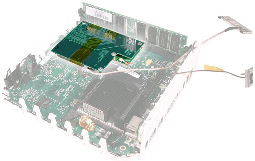
12. With your fingernail disconnect the Bluetooth antenna cable from the Bluetooth board.
