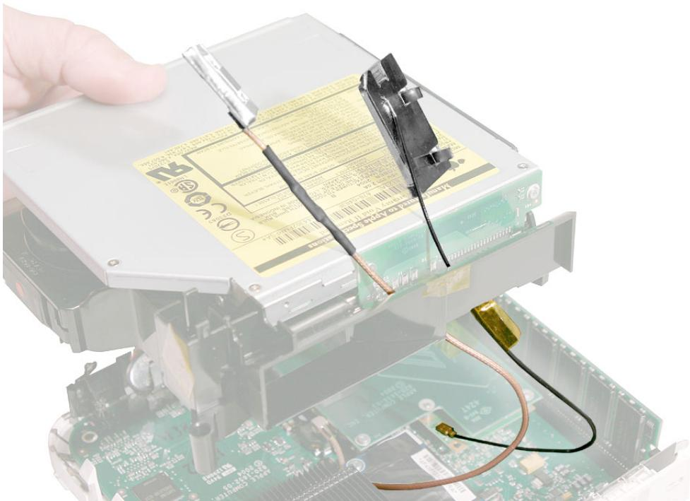
3. Lower the internal frame into place. **Note:** Route the power button cable out of the way of the internal frame.
