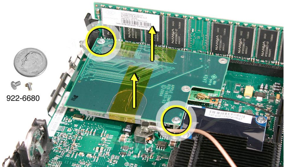
14. Turn over the mezzanine board. With a jeweler's #0 Phillips screwdriver remove the two screws on the Bluetooth board. Pull the Bluetooth board off the connector on the mezzanine board.
