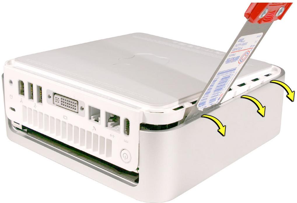
11. Push the I/O panel upward until the top housing is removed. The popping sounds will continue as you push the I/O panel; this is normal.
