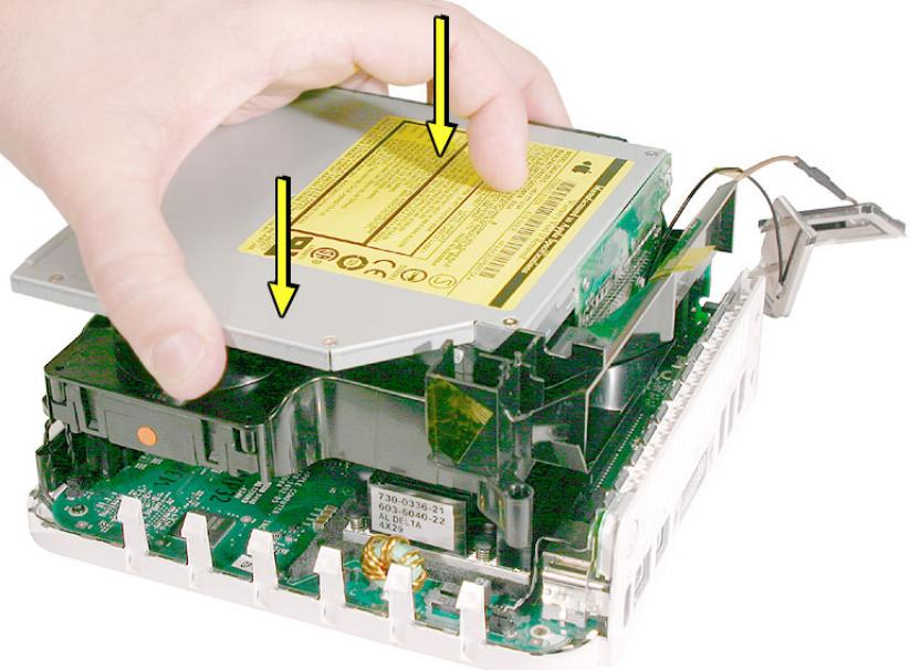
10. Route the antenna cables to the right side of the interconnect board on the internal frame as you lower the internal frame onto the logic board.**Note:** Be careful not to pinch the cables.
