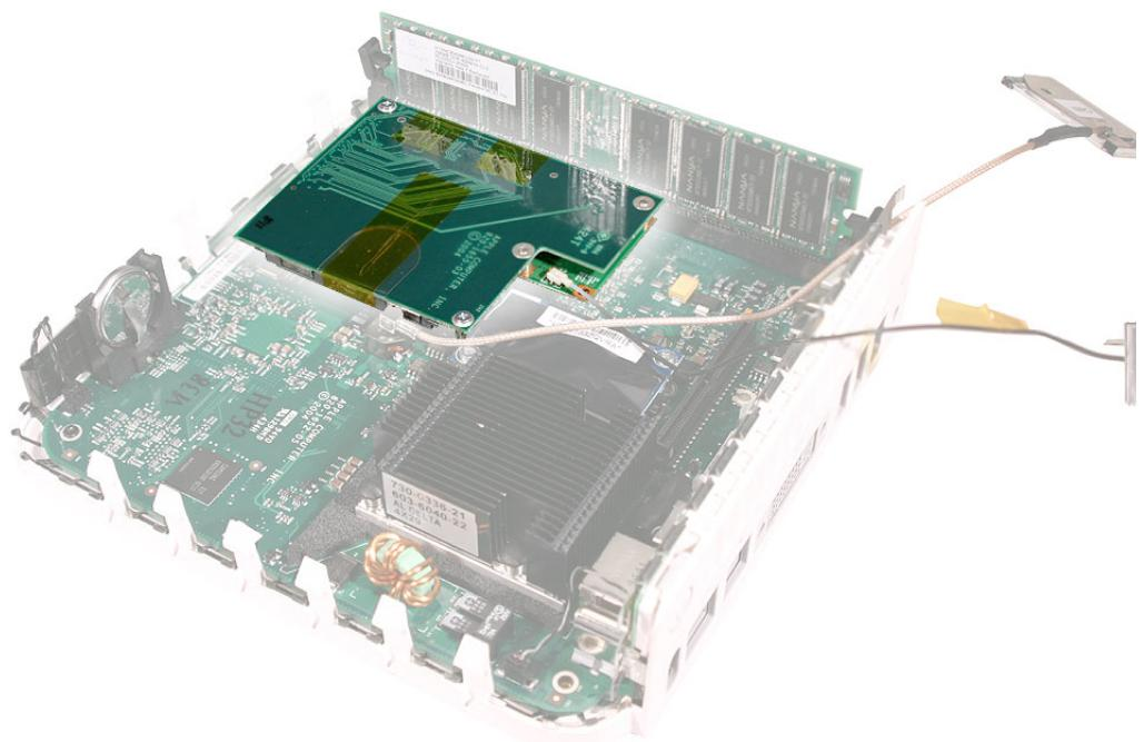
15. To access the AirPort Extreme card remove the two screws on the mezzanine board with a jeweler's # 0 Phillips screwdriver. Pull the mezzanine board straight up and off the logic board connector.
