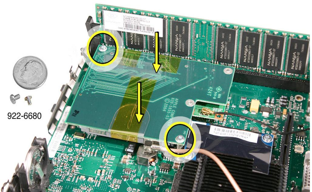
3. Make sure that the AirPort antenna cable is firmly inserted into the AirPort Extreme card. If the connector is not fully inserted, you'll see a large portion of the connector collar. For details see Knowledge Base article 108039, "Properly attaching the antenna on an AirPort Extreme card."
