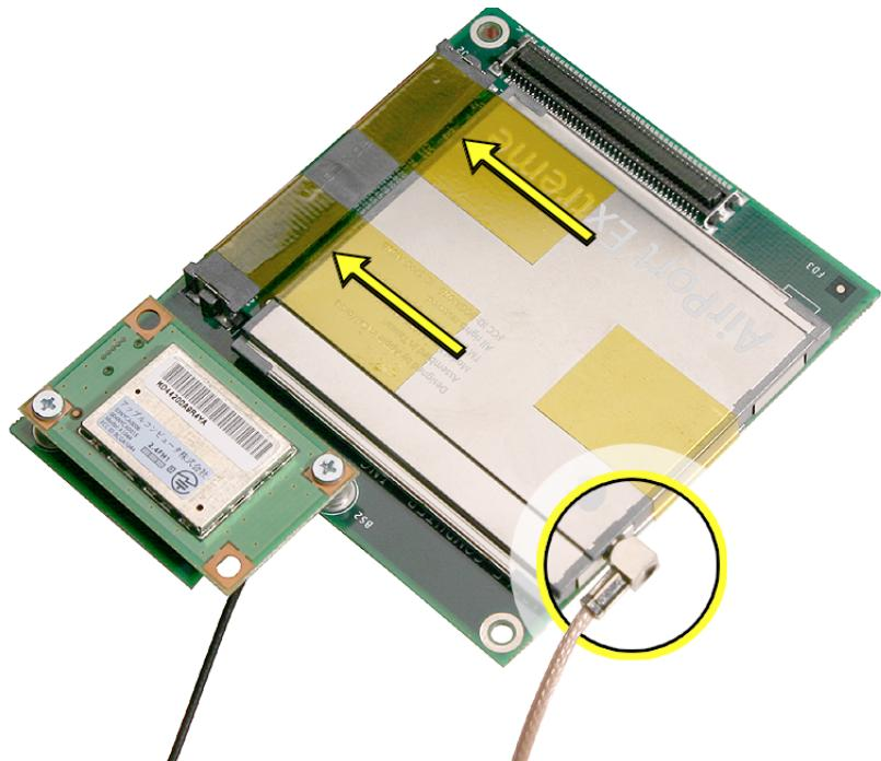
2. Turn over the mezzanine board so the AirPort Extreme card is facing down. Connect the mezzanine board to the connector on the logic board. Replace the two screws on the mezzanine board.
