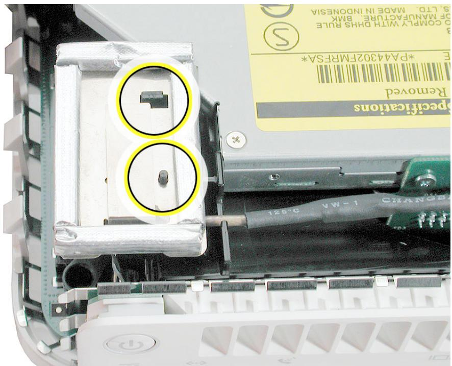
5. **Note:** The airport antenna board contained in the finished goods upgrade kit has too large a hole for the internal frames to clip onto. Use additional kapton tape to secure the antenna to the internal frame. Place a little kapton tape beneath the antenna or place a strip of tape going from the optical drive to the internal frame, where the antenna connects to the antenna board.
