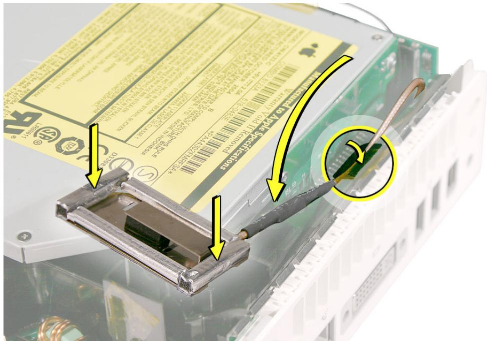
14. Lower the AirPort Extreme antenna over the black post and the clip (circled below) on the internal frame. Make sure that the AirPort antenna is not damaged or warped on the receiver end of the cable. Make sure that this end is properly seated to the internal frame (as shown below).
