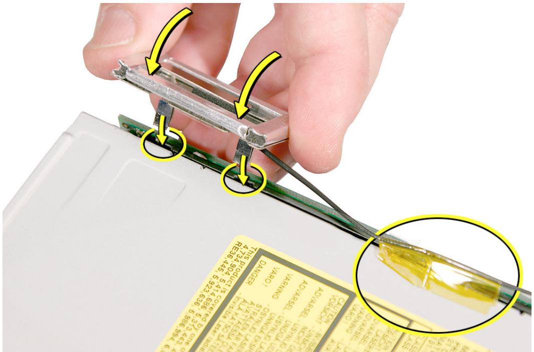
7. Replace the AirPort Extreme antenna and secure the cable with kapton tape
