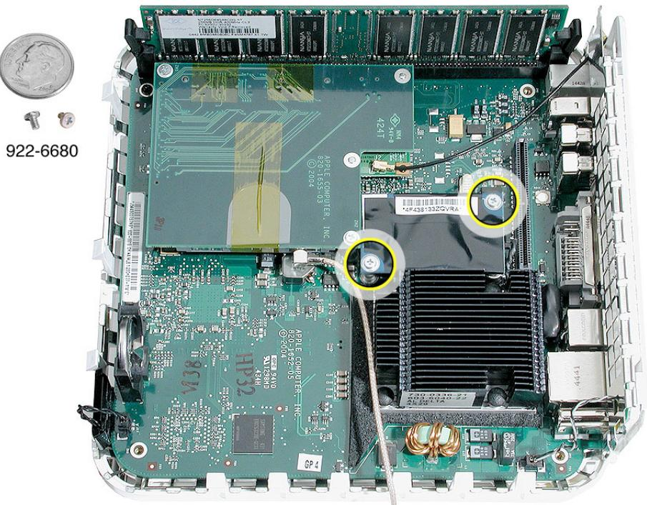
2. Using a black stick or other nonconductive nylon or plastic tool, pry the modem board off the logic board connector.
