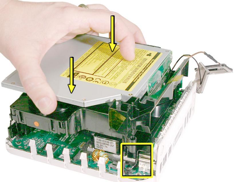
7. Route the antenna cables to the right side of the interconnect board on the internal frame. Lower the internal frame onto the logic board.
