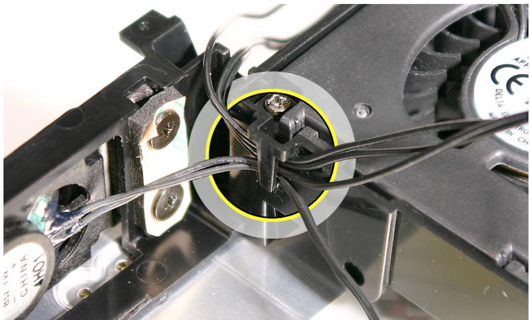
5. Route the fan cable under the clip on the outside of the internal frame.
