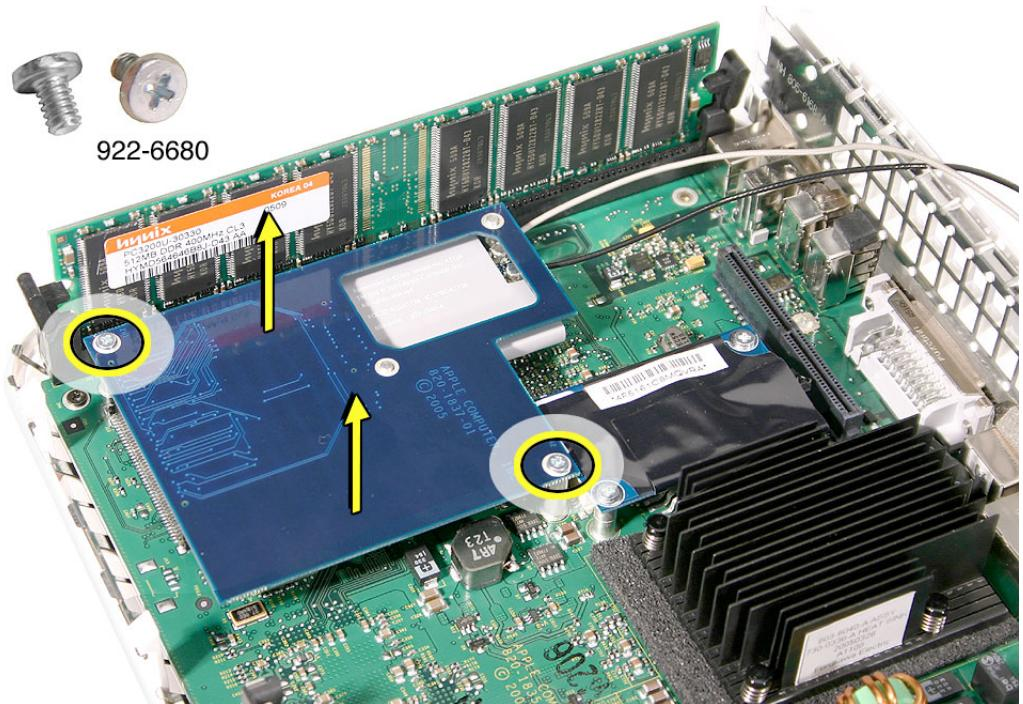
15. Turn the mezzanine board over to access the screws on the AirPort Extreme/Bluetooth card.
