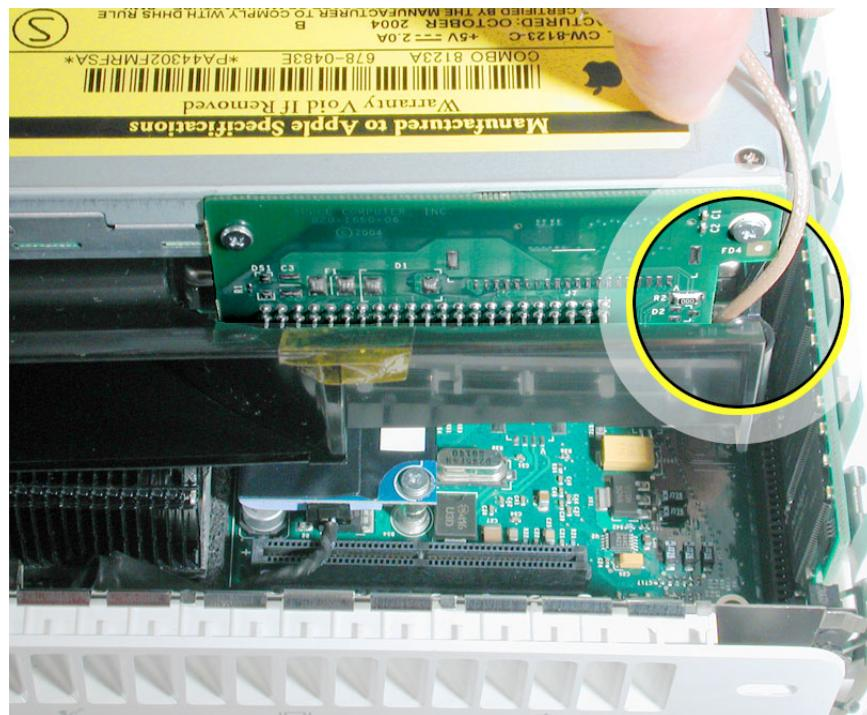
15. Replace the three screws on the internal frame.
