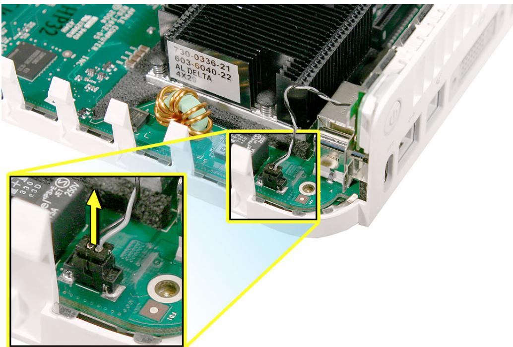
3. Using a black stick or other nonconductive tool, disconnect the LED cable from the connector on the logic board. **Note:** This connector is very small. Don't pull on the cable; pull on the connector.
