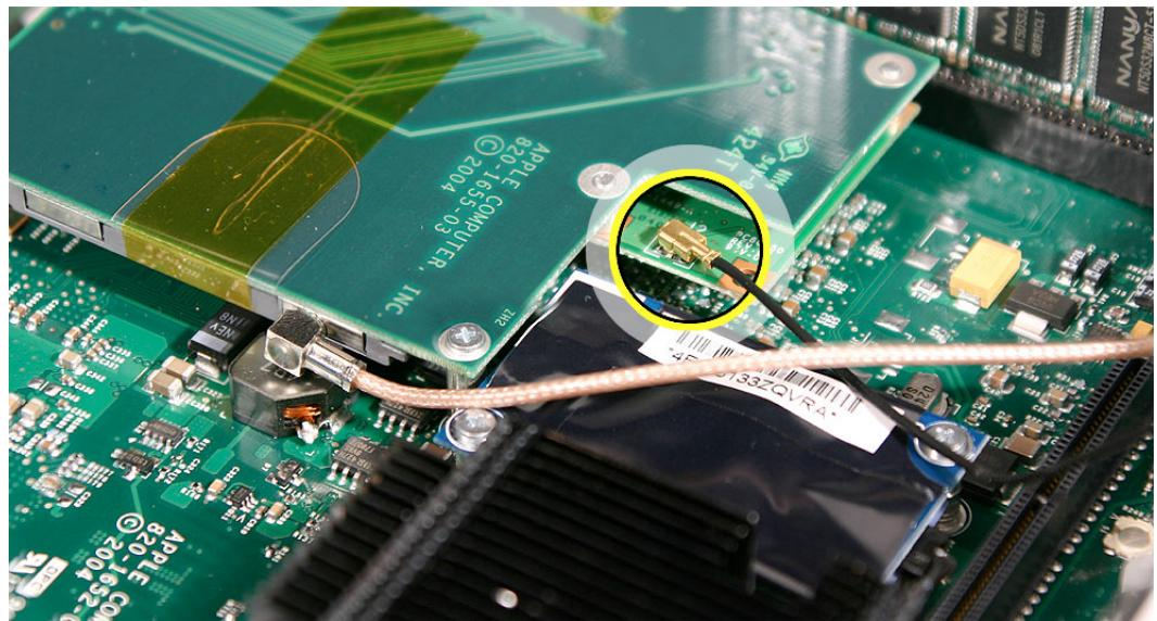
3. Make sure that the mezzanine board is properly seated on the logic board.
