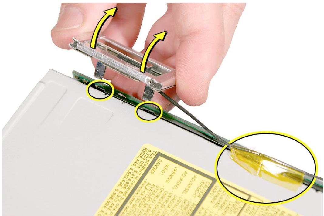
4. Set the Bluetooth antenna off to the side and out of the way. **Note:** The Bluetooth board and antenna cable are connected to the mezzanine board located under the internal frame.
