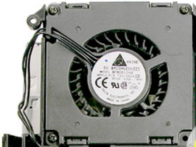
2. Place the fan in the internal frame.
