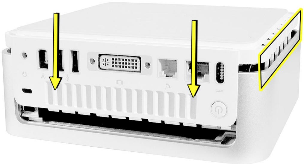
2. Squeeze the unit together firmly as shown. Proceed to the next step.
