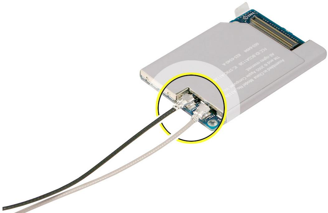
2. Connect the AirPort Extreme/Bluetooth card to the mezzanine board. Replace the two screws on the AirPort Extreme/Bluetooth card.
