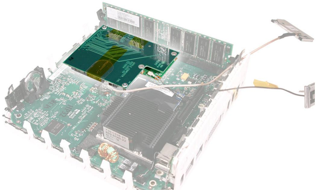
4. Reassemble the computer and test. Again, depending on the Mac mini model, if the AirPort Extreme card is still not recognized, test with a known good AirPort Extreme card or AirPort Extreme/Bluetooth card. If the known good card is recognized, replace the AirPort Extreme card or the AirPort Extreme/Bluetooth card.
