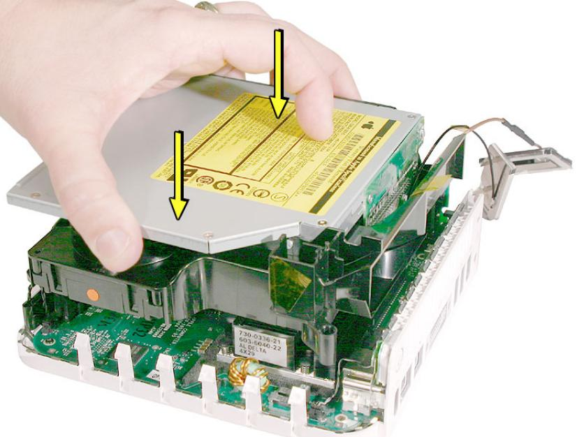
22. Route the antenna cables to the right side of the interconnect board on the internal frame as you lower the internal frame onto the logic board. **Note:** Be careful not to pinch the cables.
