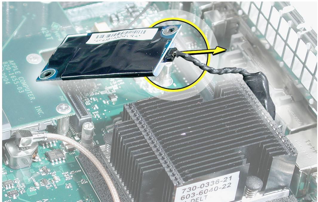
2. Turn over the logic board. Using a black stick, push the RJ-11 connector off the logic board.
