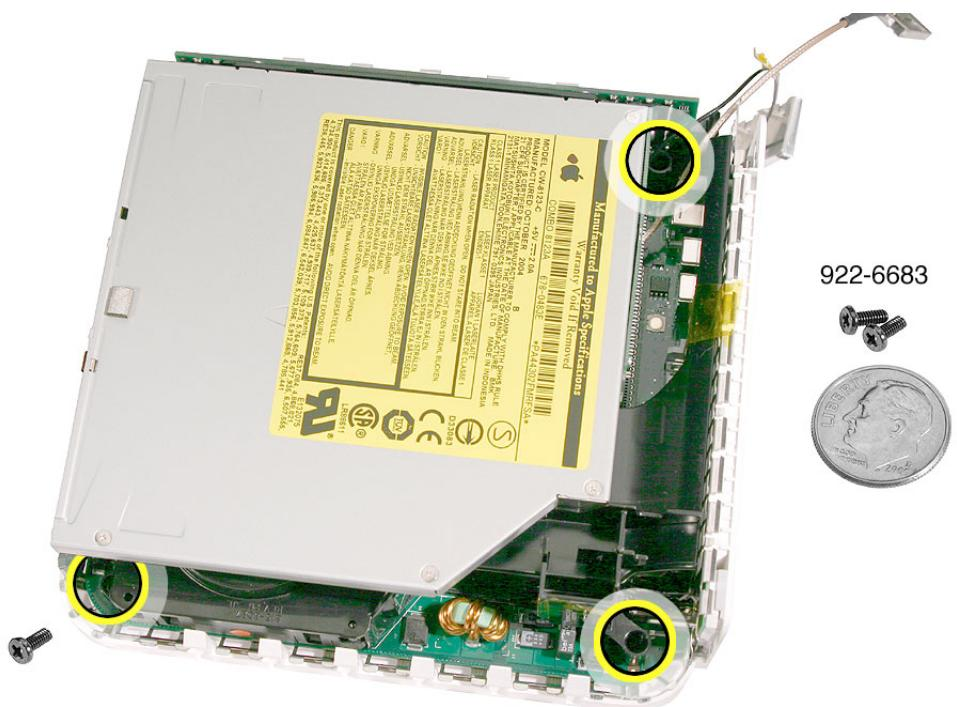
10. Lift the internal frame straight up.
