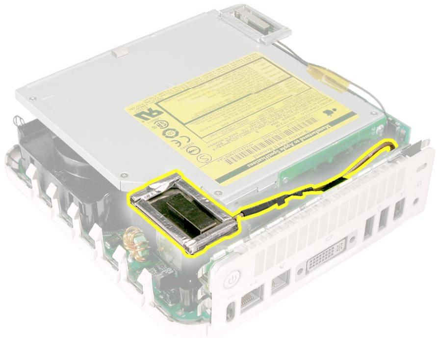
2. Using a black stick, push the black latch (see inset) toward the I/O ports to release the antenna from the internal frame.
