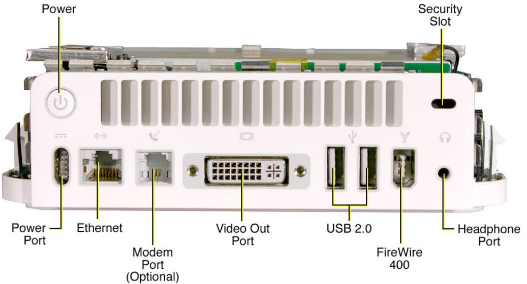
The Mac mini ports shown with the modem plug in place.
