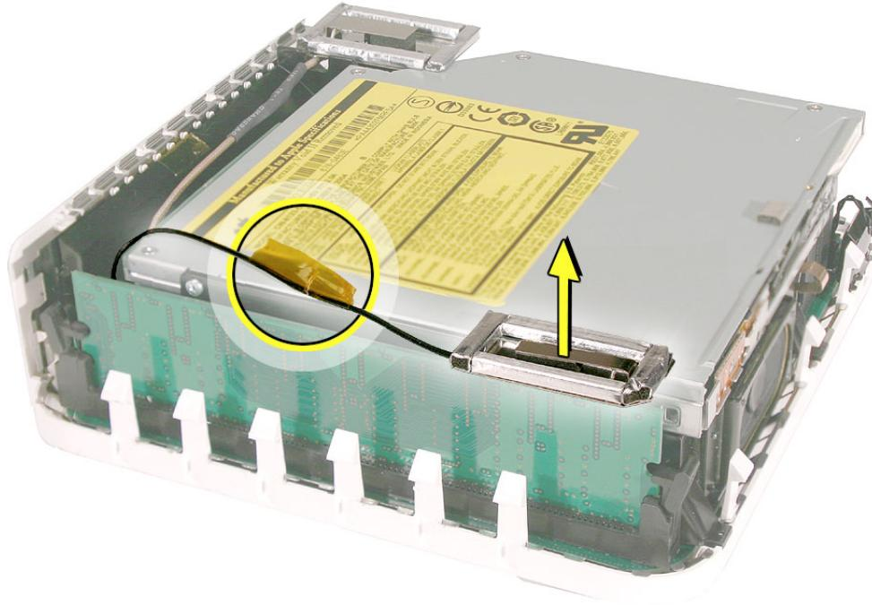
2. To release the memory from its slot, push down on the two side latches. Then pull the memory module out of the slot. **Caution:** Be careful that the latch on the left doesn't damage the EMI clip near the I/O port.
