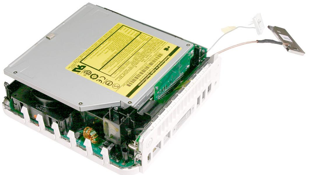
6. Free the power button cable from the kapton tape on the internal frame.
