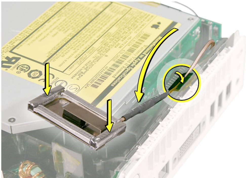
10. Gently fasten the antenna onto the internal frame. The antenna is held in place by the black clip and black post (shown below).
