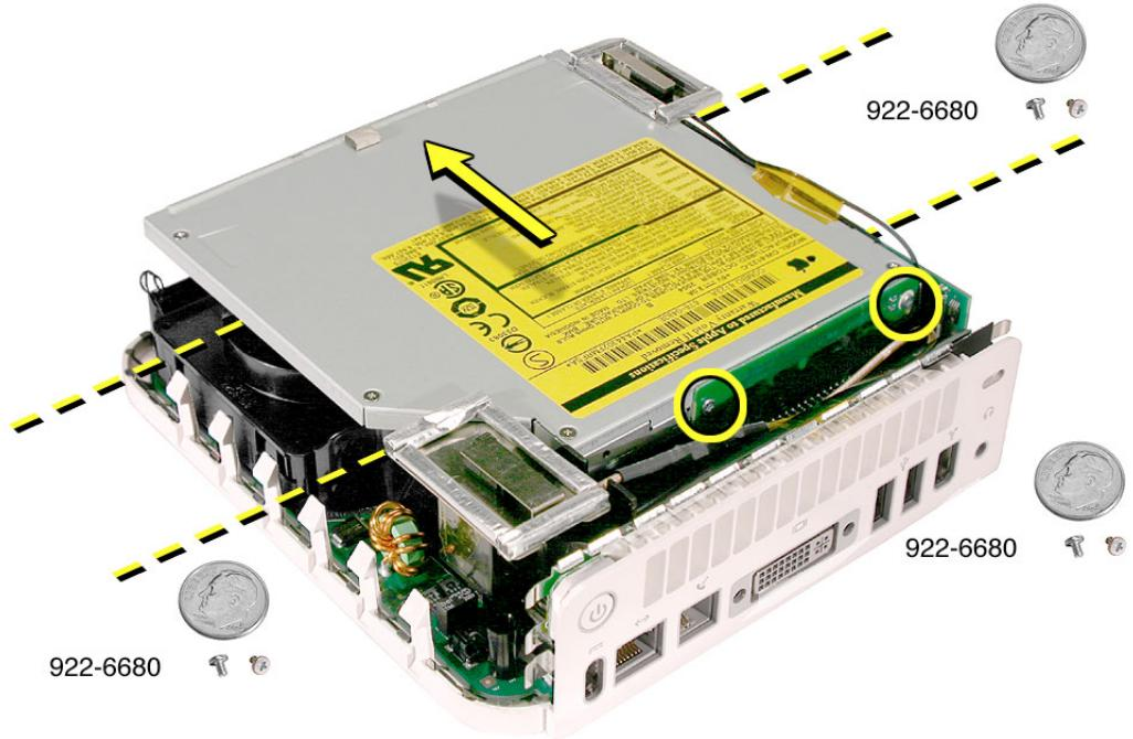
2. Using a black stick, pry the optical drive off the interconnect board (#1) and slide the optical drive (#2) off the internal frame.
