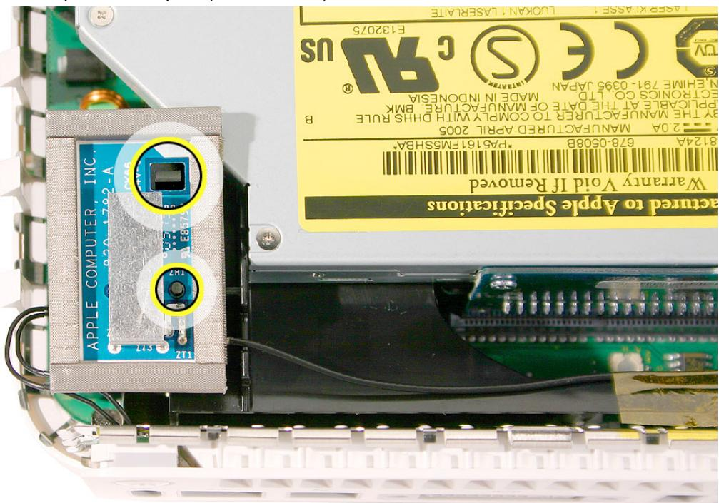
12. Secure the power button cable to the internal frame with the kapton tape.
