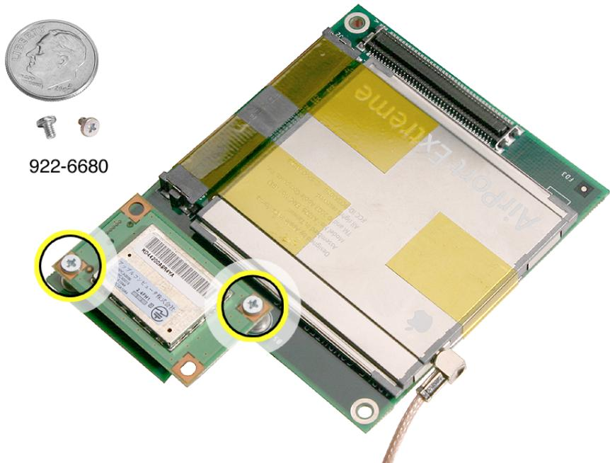
2. Connect the mezzanine board to the logic board. With a jeweler's #0 Phillips screwdriver replace the two mezzanine board screws.
