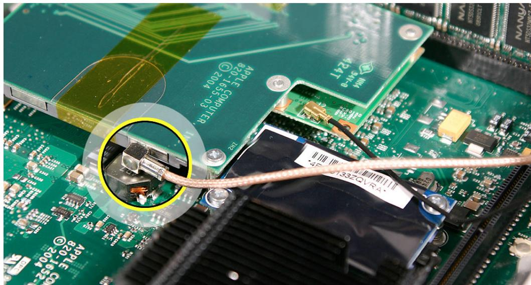
4. Hold the internal frame over the logic board as shown. Route the AirPort and Bluetooth antenna cables up through the opening in the internal frame.
