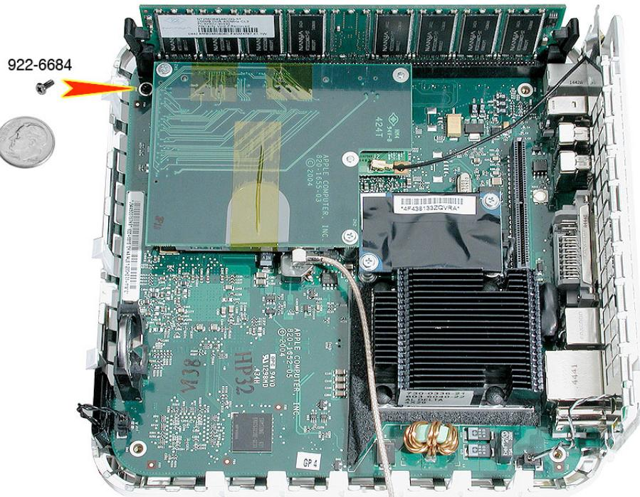
2. Disconnect the power-on cable from the connector on the logic board.
