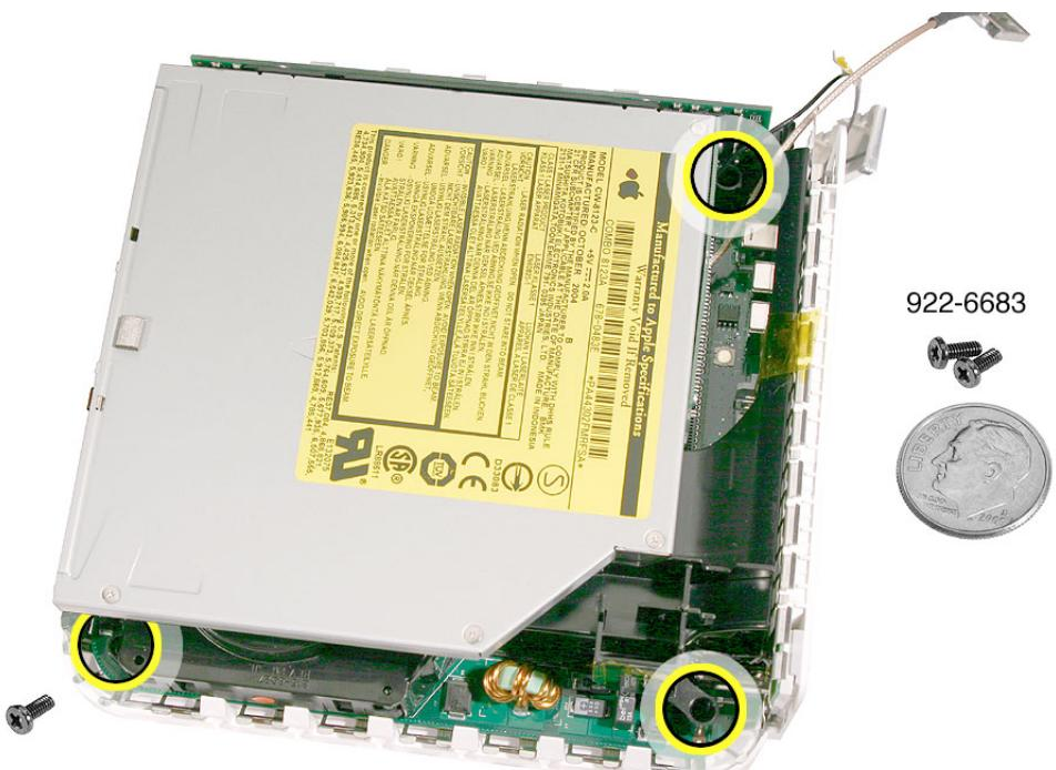
9. Replace the Bluetooth antenna. Secure the antenna cable with kapton tape.
