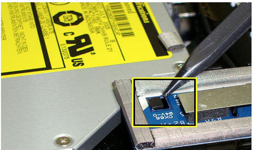
28. Secure the power button cable to the internal frame with the kapton tape.
