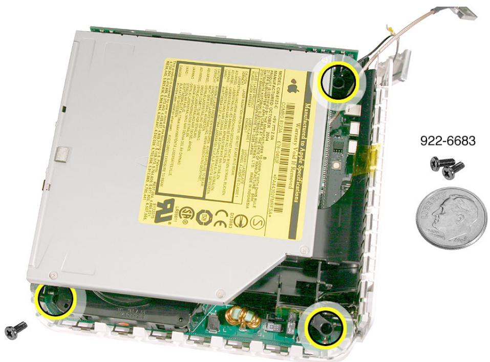
11. Lift the internal frame straight up.
