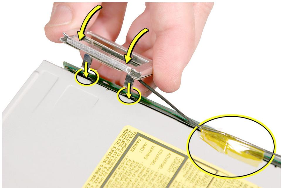
10. Replace the AirPort Extreme antenna. Secure the cable with kapton tape. **Important:** Take care handling the AirPort antenna as a bent or warped antenna will affect AirPort connectivity.
