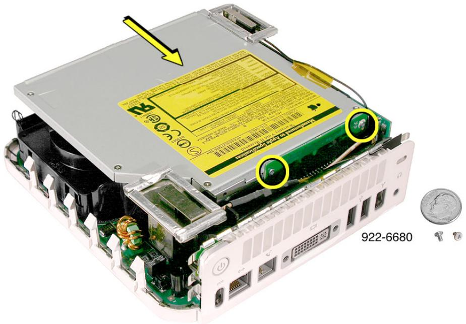
2. **Note:** If you are installing a replacement drive, install the EMI gasket (that came with the replacement optical drive) on the top and center of the optical drive.
