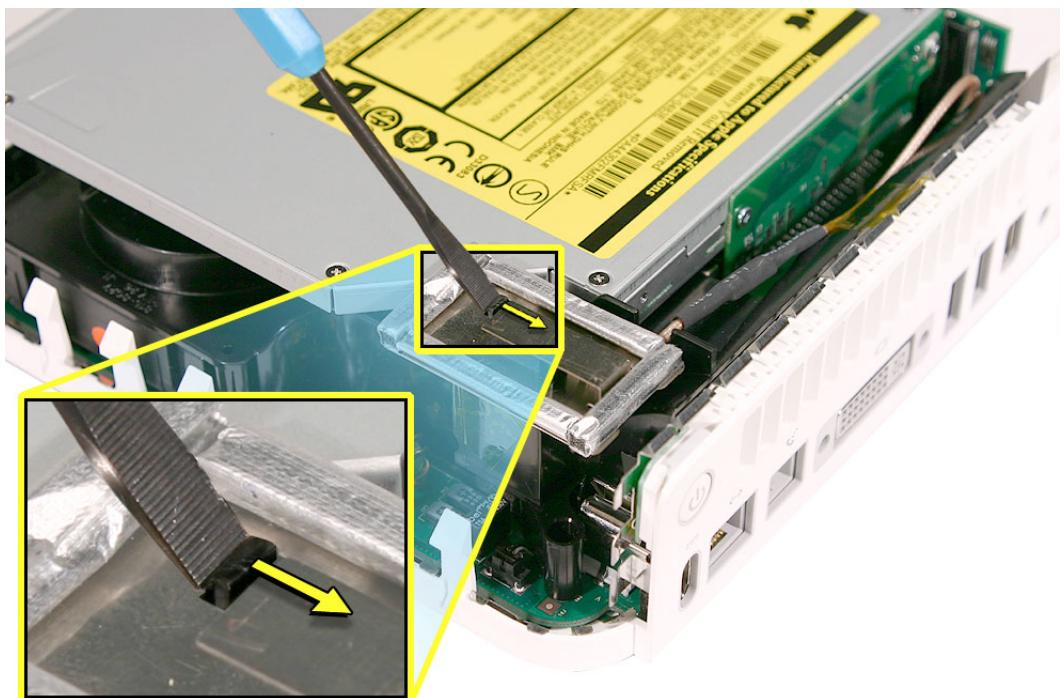
7. Carefully lift the antenna off the frame. Free the antenna from the kapton tape (circled). **Important:** Take care handling the AirPort antenna as a bent or warped antenna will affect Airport connectivity
