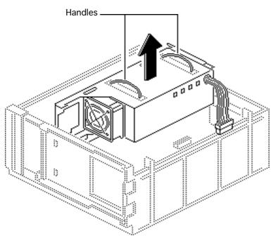
4 Note: If you are servicing a Workgroup Server 9150/120, you must disconnect the processor fan from the logic board before removing the power supply. The processor fan attaches to the underside of the power supply.
