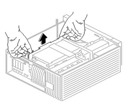
**Caution:** In the next step, pull up evenly on both sides of the card to avoid bending the connector pins.
