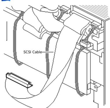
26 Attach the end of the five-drive SCSI cable to the internal SCSI connector on the logic board.
