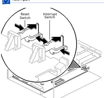
Press in on the sides of the interrupt and reset switches and push them out of the case.
