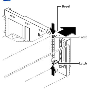
3 Release the two plastic latches on the inside of the CD-ROM bezel and remove the bezel.
