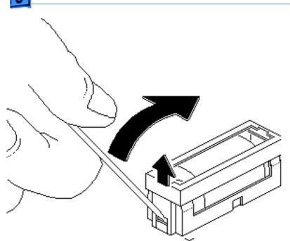
Using a small flat-blade screwdriver, pry open the latch at the end of the battery holder and lift off the cover.
