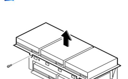
1 Remove the two screws that secure the top of the drive carrier to the bottom of the drive carrier.
