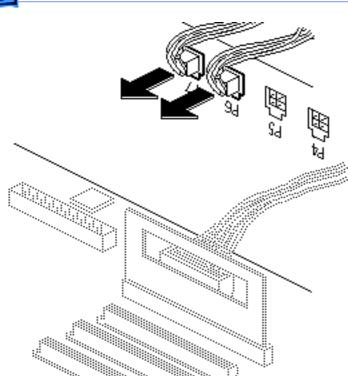
Disconnect the tape drive and CD-ROM drive power cables from the power supply.
