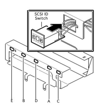
3 There are five openings in the bottom panel of the drive carrier for the SCSI ID switches. The openings are labeled A-E.
