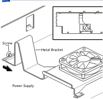
Replacement Note: The processor fan attaches to the middle of the power supply on the underside. Position the fan bracket at a 90 degree angle to the power supply. Insert the two tabs on the bottom of the bracket into the metal slots on the power supply. Lay the fan and bracket flat against the power supply and push the end of the metal bracket under the screw that secures it to the power supply.
