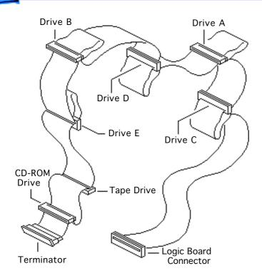
The SCSI cable connects up to five hard drives and one tape drive. The illustration on this page indicates which connectors attach to which peripherals. The pull tabs on the cable are marked as illustrated.
