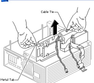
4 **Note:** In this step, be careful that none of the cables catch on the case.
