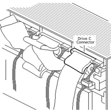
25 Fold over the cable and attach the drive C connector to the drive in slot C.
