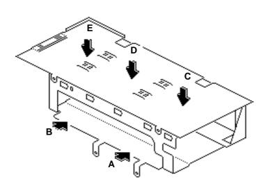
Note: Hard drives must be installed in the five-drive carrier in the order shown. If you install fewer than five drives, you must still install the drives in the order shown.
