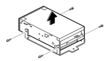
3 Remove the four screws that secure the tape drive to its carrier and lift up on the tape drive to remove it.
