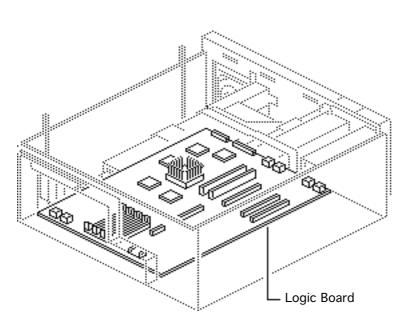
**Note:** When returning the logic board to Apple, return it with the ROM SIMM and terminator card (located in the Power Macintosh video slot) installed, but remove the cache and DRAM SIMMs before returning the board.
