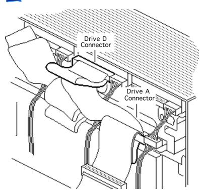
23 Attach the drive D connector on the fivedrive SCSI cable to the hard drive in slot D.
