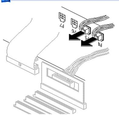
Disconnect the SCSI power cable(s) from the power supply.
